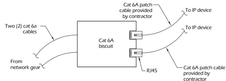
DETAIL NOT TO SCALE **6** WIRELESS ACCESS POINT TYPICAL ETHERNET BISCUIT
