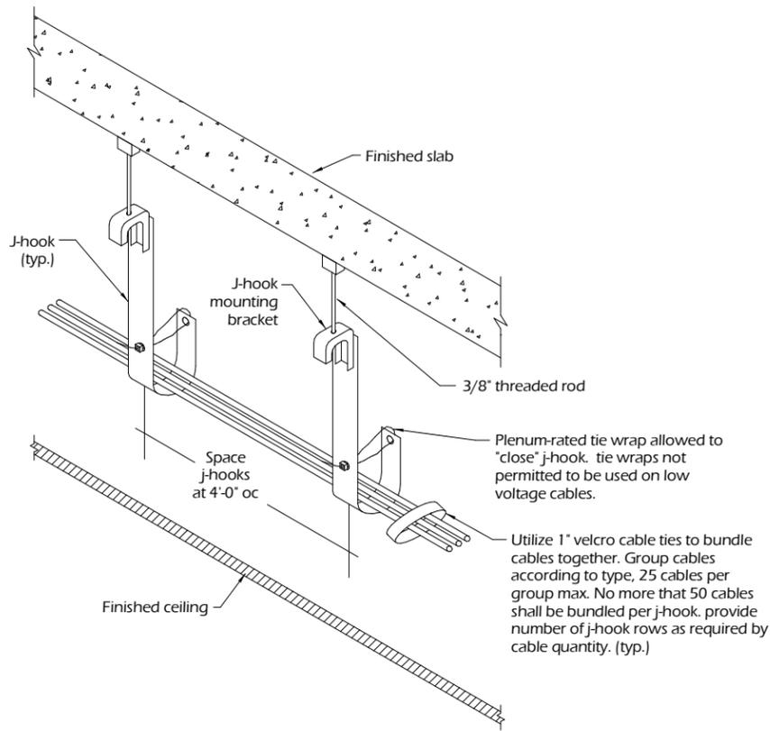
DETAIL NOT TO SCALE **1** ACCESSIBLE CEILING CABLE INSTALLATION DETAIL
