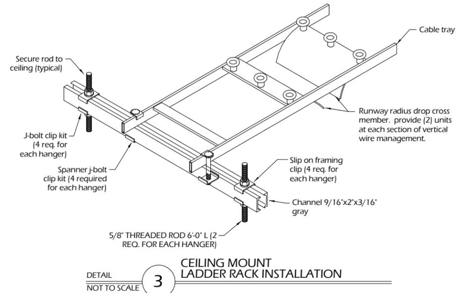
DETAIL NOT TO SCALE **3** CEILING MOUNT LADDER RACK INSTALLATION
