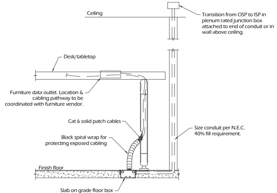
DETAIL NOT TO SCALE **2** FLOOR BOX FURNITURE FEED DETAIL MOUNTED IN SLAB ON GRADE
