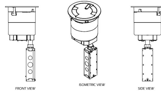
2 FLOOR BOX - BASIS OF DESIGN - POKE - THROUGH TYPE (WIREMOLD 8ATC)
