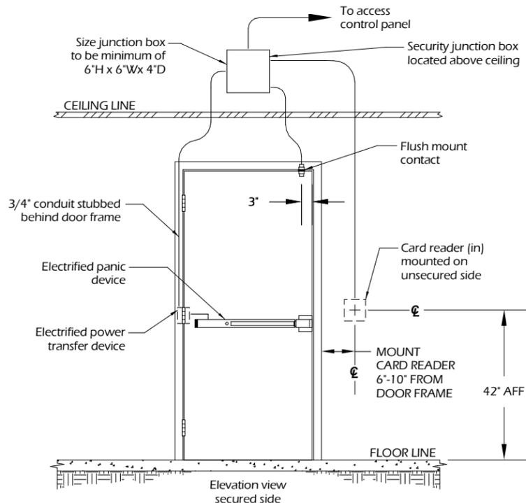
Single door with card reader, door contact, electrified panic device, power transfer device
