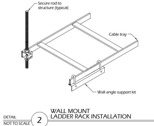
DETAIL NOT TO SCALE **2** WALL MOUNT LADDER RACK INSTALLATION
