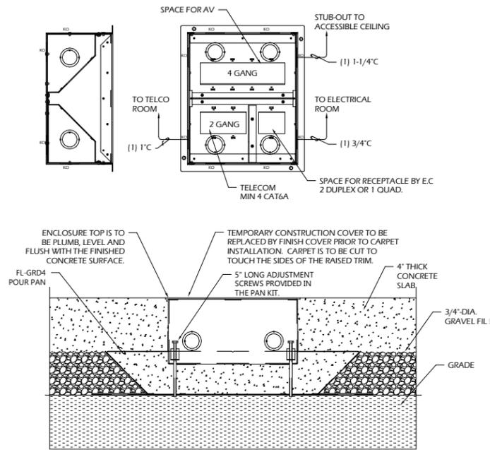
1 FLOORBOX - CONCRETE FLOOR - BASIS OF DESIGN (FSR FL-500P-6)
