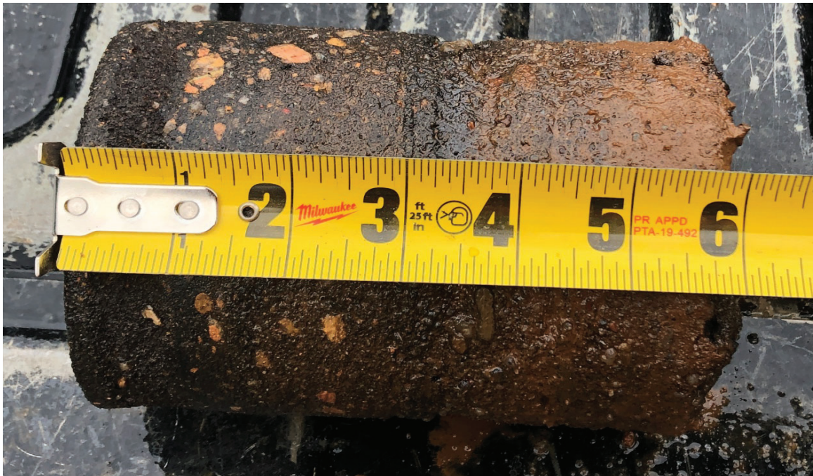
Core SW-02 - Westbound lane, Measured Thickness of 6 inches
