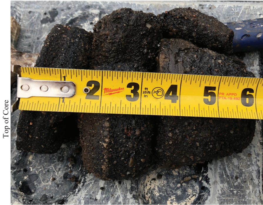
Core SW-03 - Eastbound lane, Recovered Thickness of 5.5 inches, 9 inches cored, Completely Stripped asphalt 3.5 to 6.5 inches.
