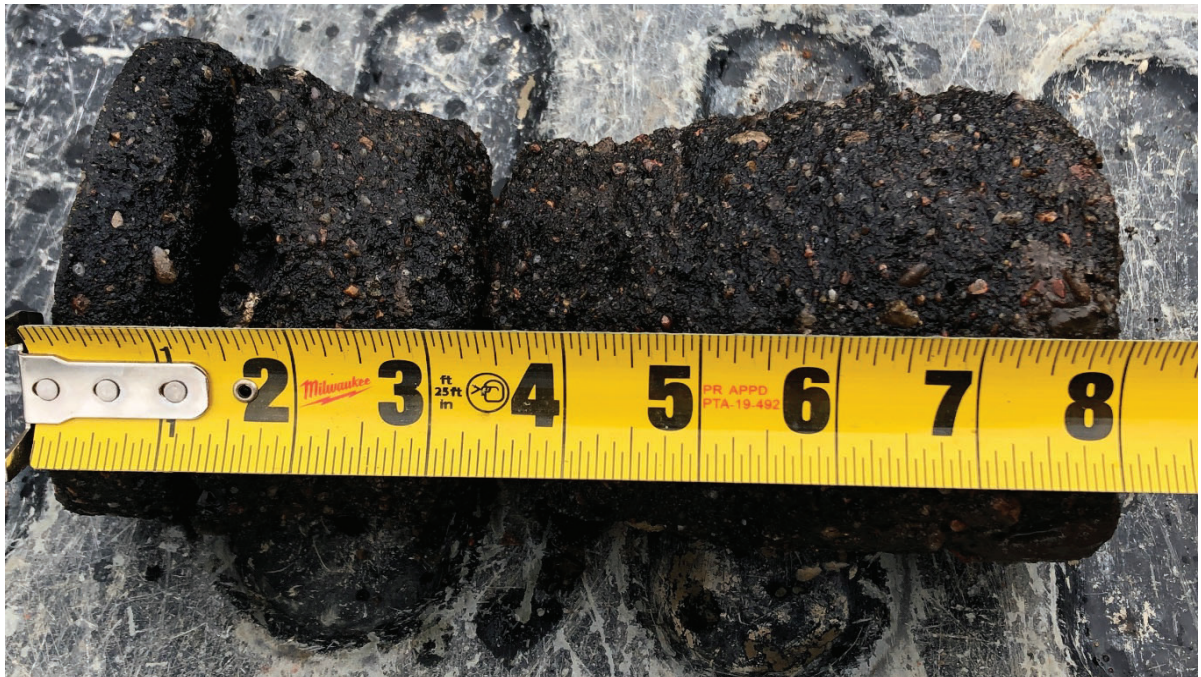
Core SW-05 - Eastbound lane, Measured Thickness of 8 inches
