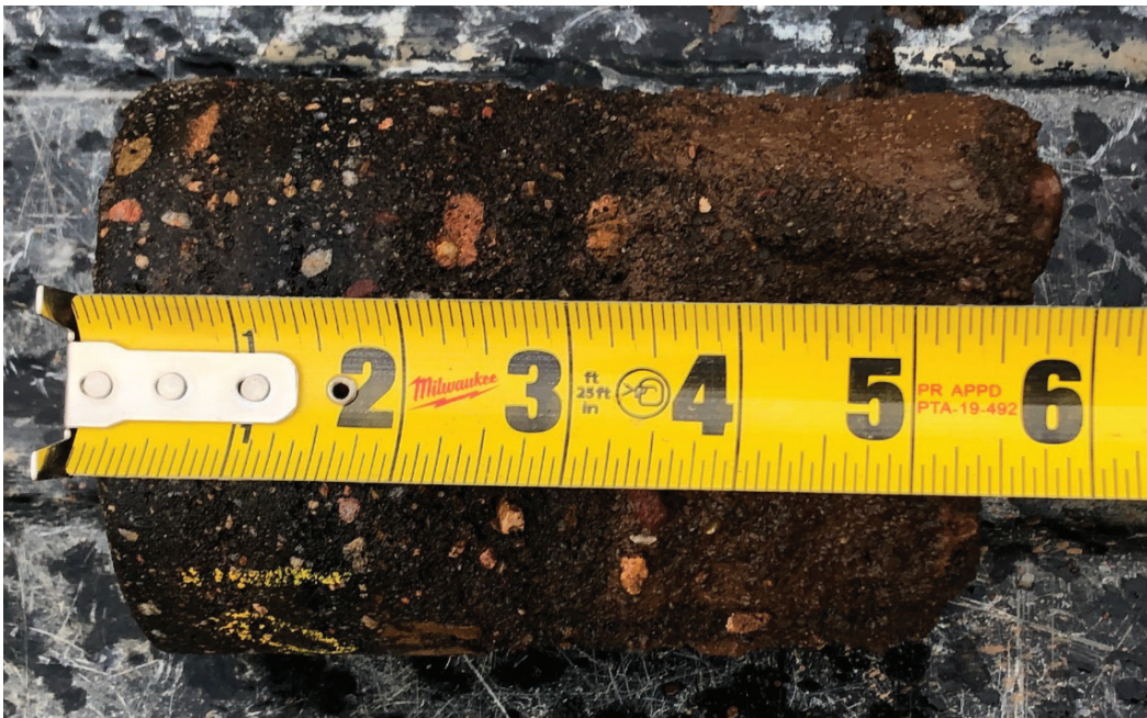
Core SW-01 - Eastbound lane, Measured Thickness of 5-1/2 inches
