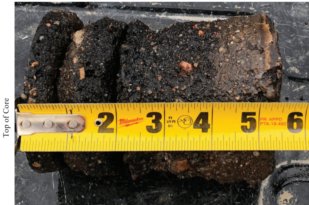
Core SW-04 - Westbound lane, Measured Thickness of 5 inches
