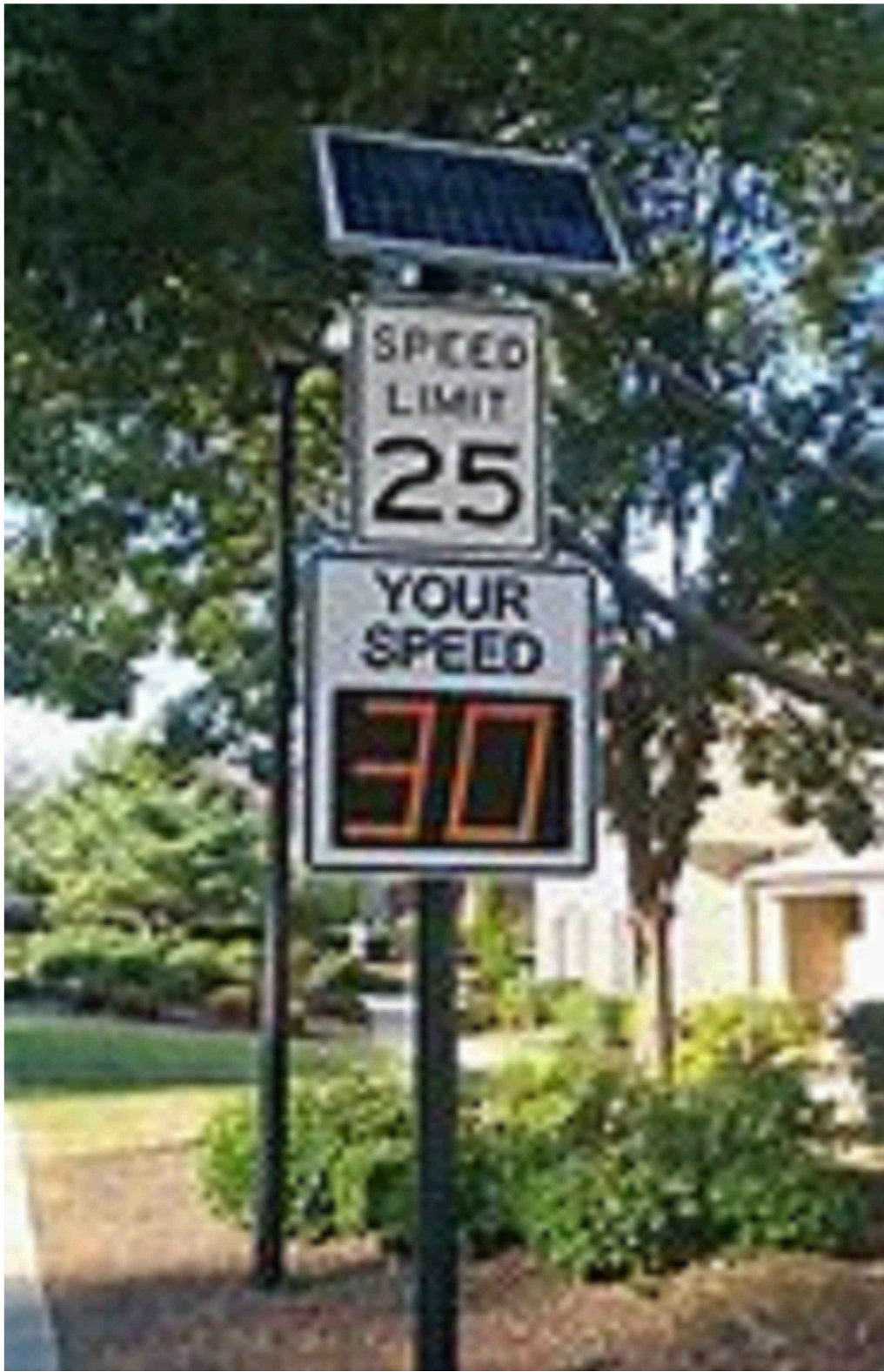
Figure 2. Solar Powered Radar Speed Limit Sign
