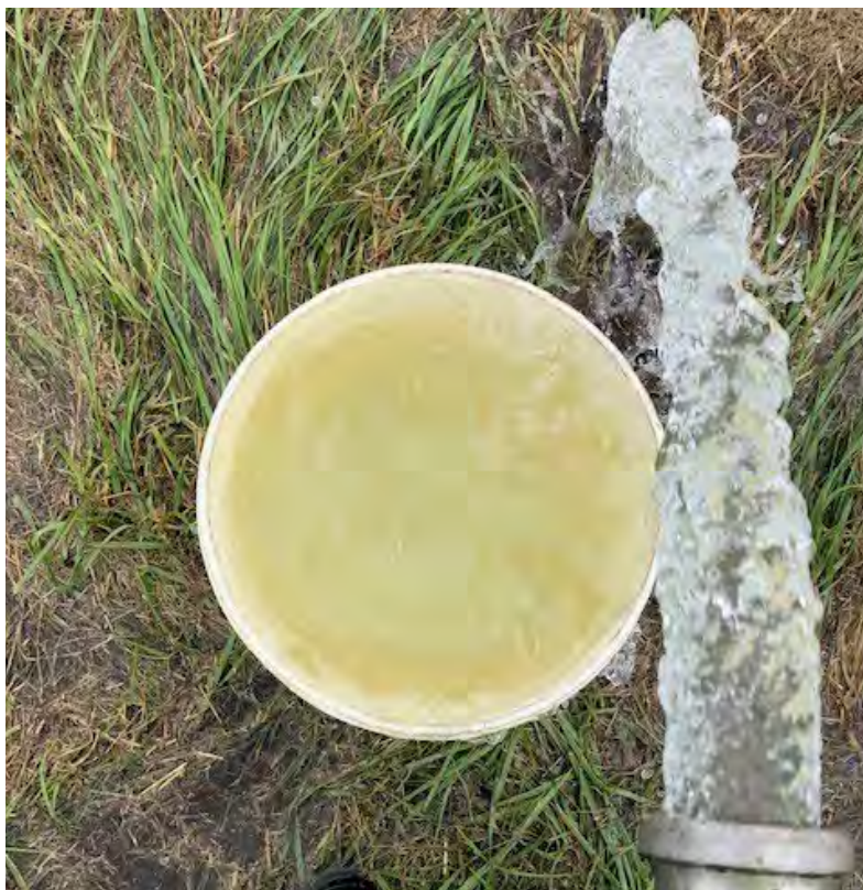
Figure 12: Final discharge water at the end of post-surge airlifting (RW-68)
