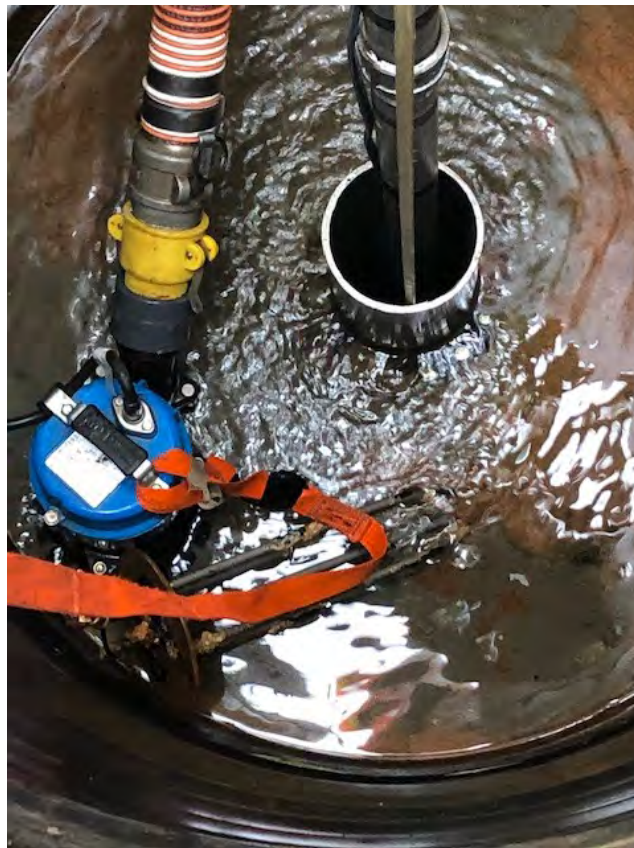
Figure 8: Groundwater flowing around well riser pipe at base of manhole vault during capacity testing in relief well RW-67B
