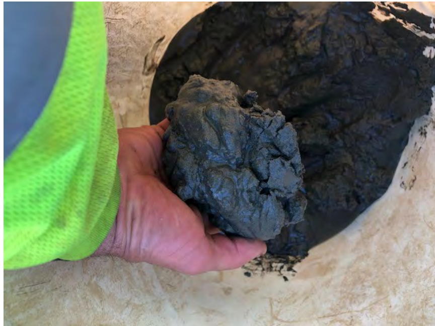
Figure 10: Airlifted material (post-surge) from relief well-68A
