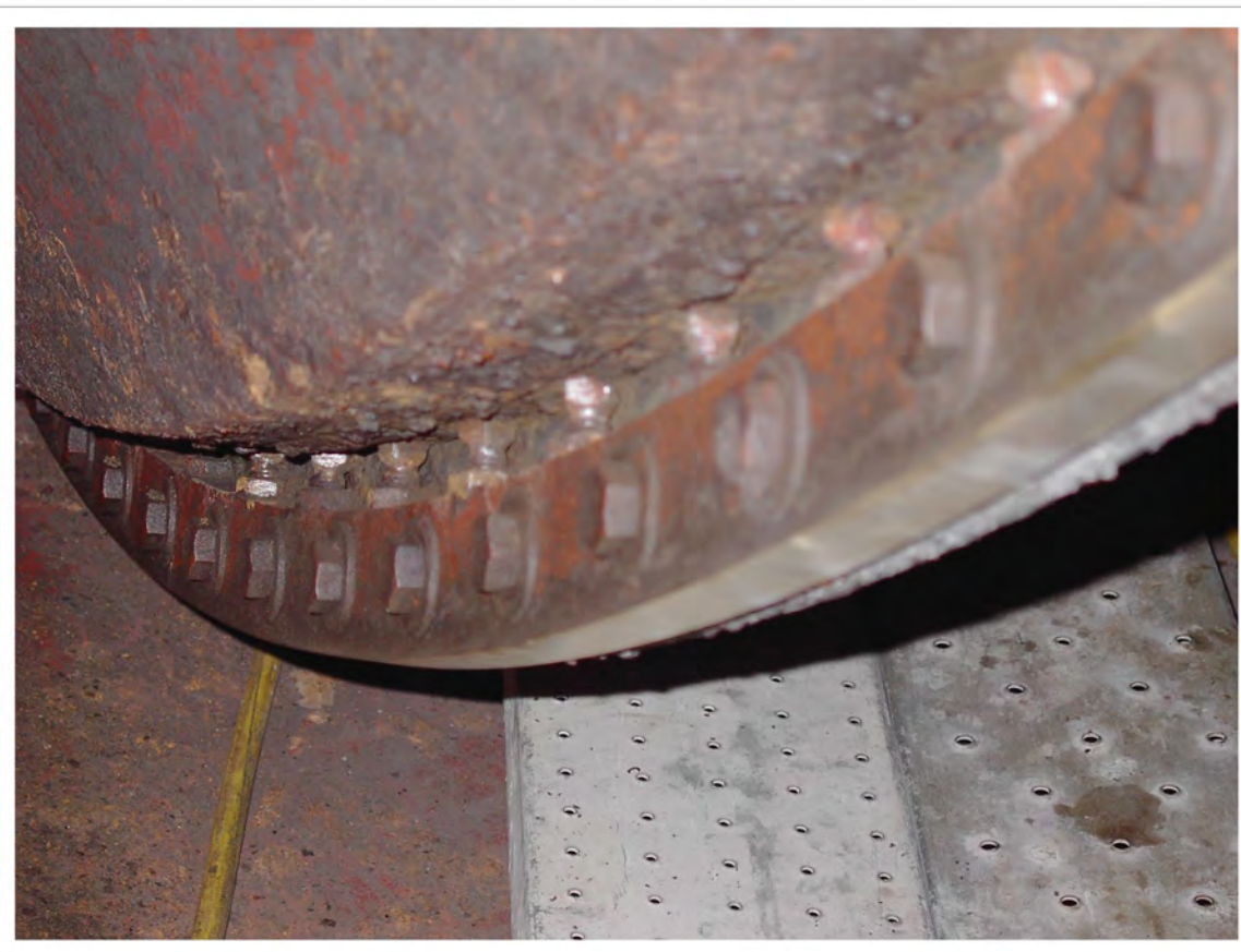
CLOSE-UP OF VALVE DISC BRONZE SEAL
