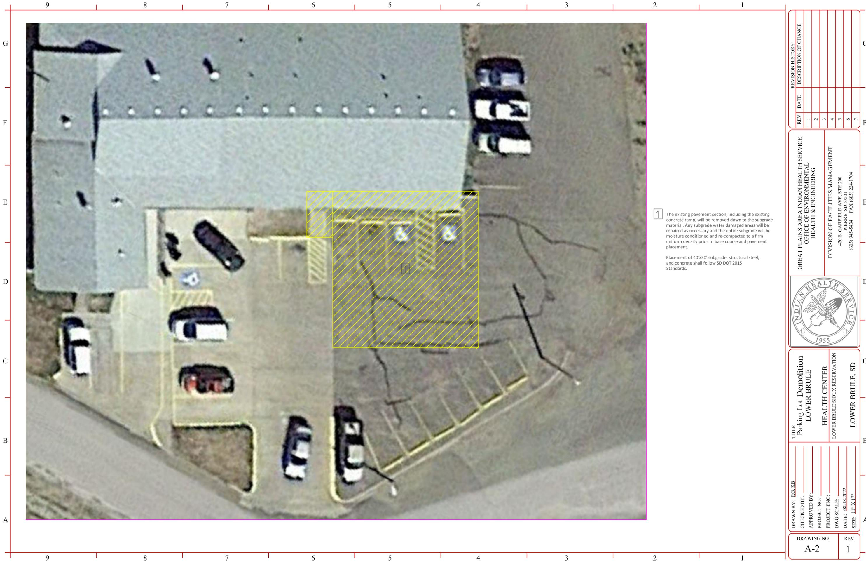
**1** The existing pavement section, including the existing concrete ramp, will be removed down to the subgrade material. Any subgrade water damaged areas will be repaired as necessary and the entire subgrade will be moisture conditioned and re-compacted to a firm uniform density prior to base course and pavement placement.
