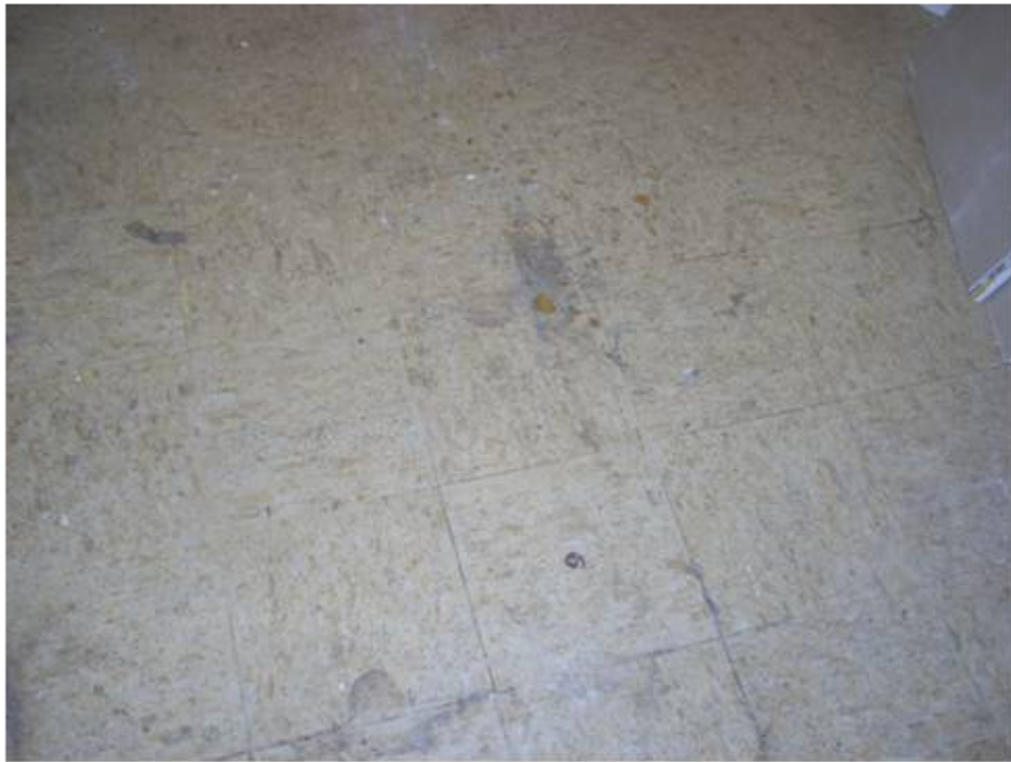
12"x12" Tan Floor Tile and Mastic, Samples 31A and 32A
