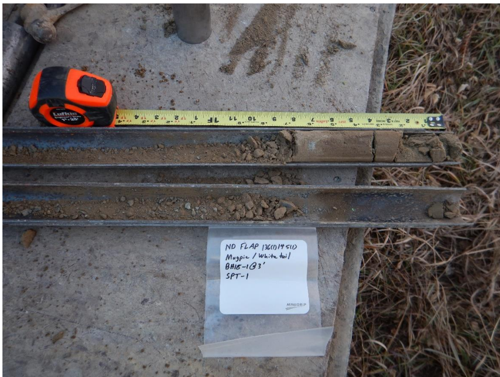
Photo 2:- Borehole BH18-01, SPT-1
