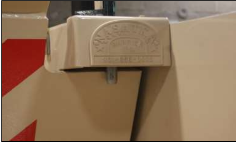
Figure 31. Gate Plate Locked In Place
