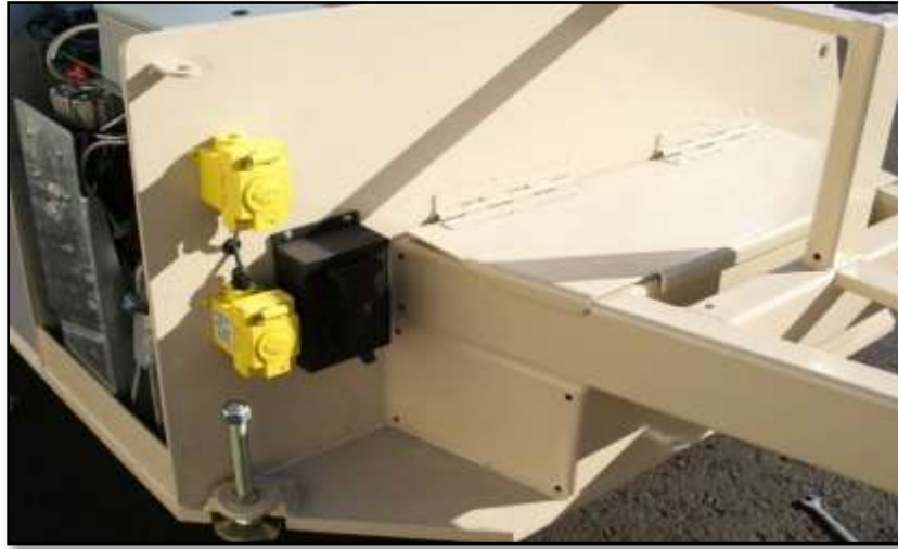
Figure 32. Tether Control Pendant Connection
