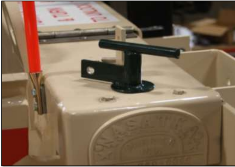
Figure 35. Locking Pin Secured
