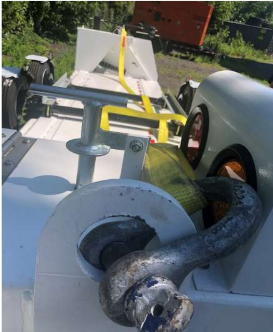
Figure 3. Hoisting Strap Locations
