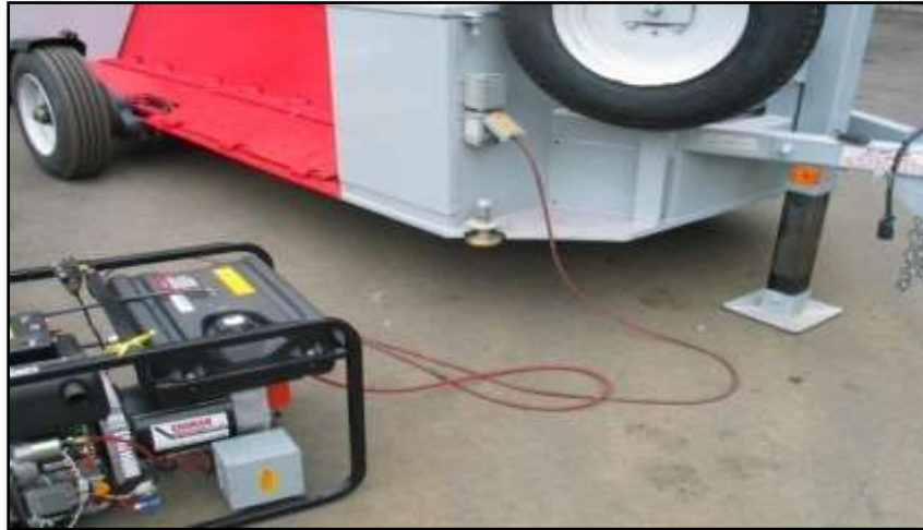
Figure 33. Connecting A Generator To The Barrier
