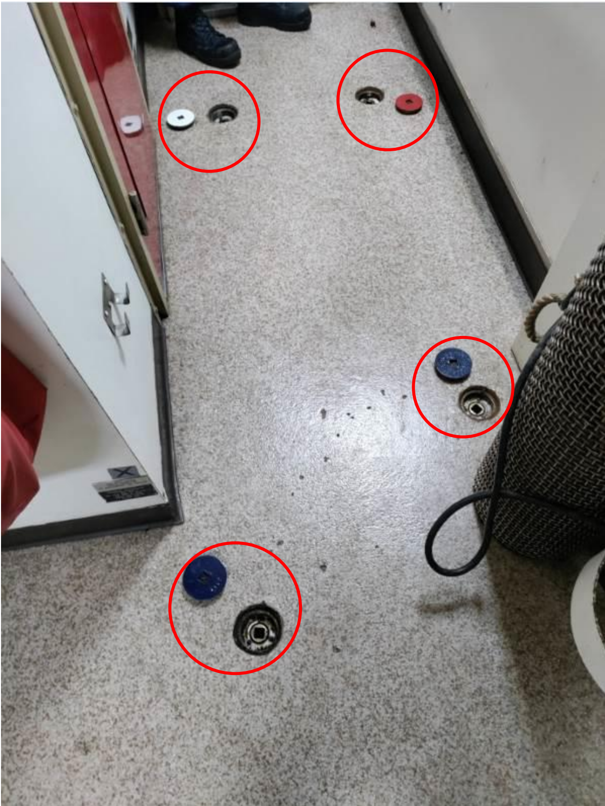
FIGURE 2 – EXAMPLE OF DECK BOXES ON INSIDE SUPERSTRUCTURE
