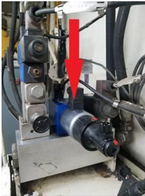
FIGURE 1. DCV TO BE REMOVED
