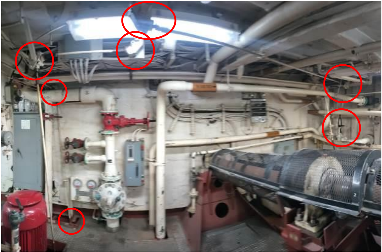
FIGURE 4 – EXAMPLE OF REMOTE VALVE OPERATORS IN ENGINE ROOM
