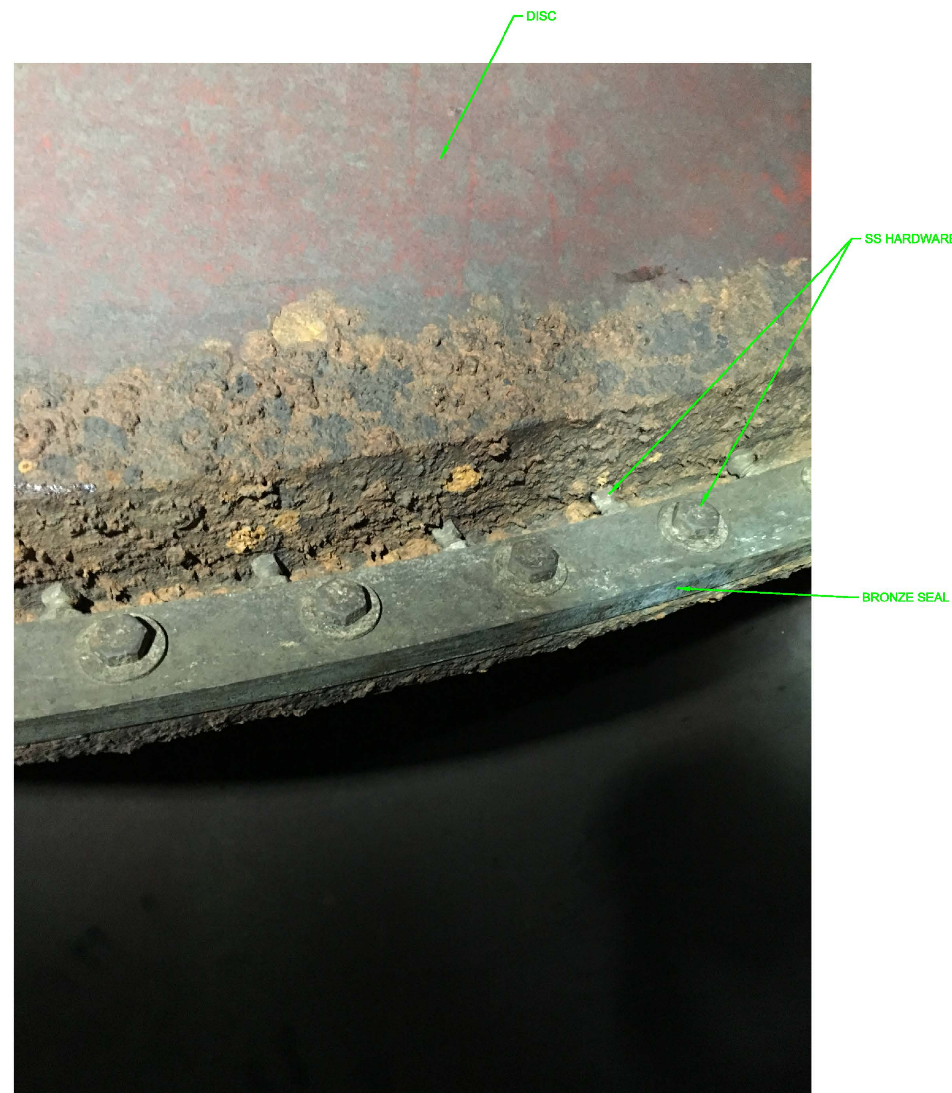
" PICTURE 4 - UNIT 4 BUTTERFLY VALVE DISC BRONZE SEALS "
