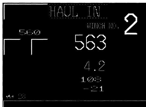
Screen No. 8 Operation menu, Haul in mode.
