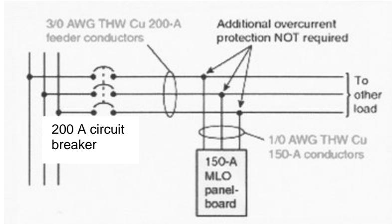
**The 1/0 AWG tap conductors cannot exceed 10' in length**
