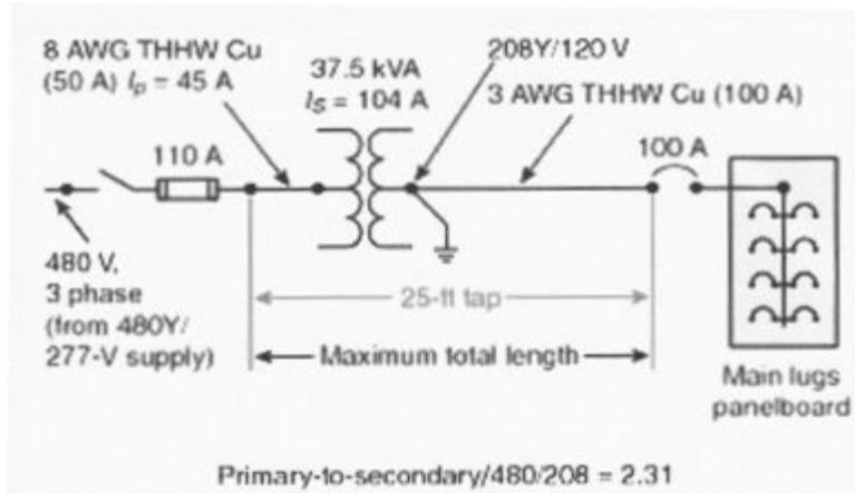
(3) NEC 240.21(B)(3) Taps supplying a transformer with primary plus secondary not over 25 feet long:
