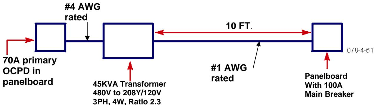
(1) NEC 240.21(C)(2) Transformer secondary conductors supplying a single load or each set of conductors supplying separate loads, shall be allowed without an OCPD as follows:
