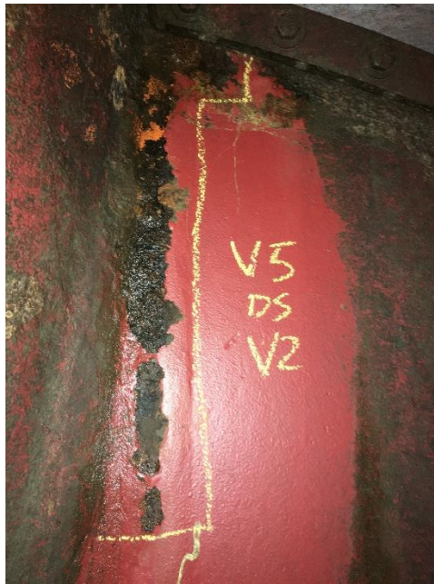
Figure 2.3: Example cleaned surfaces on Valve 5 downstream weld V2.
