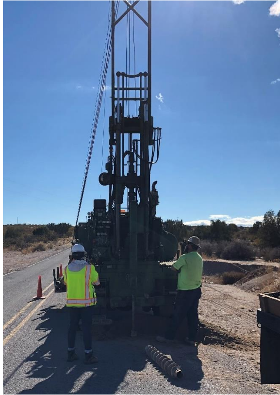
Photo 103: BH21-06, Hollow Stem Auger Drilling
