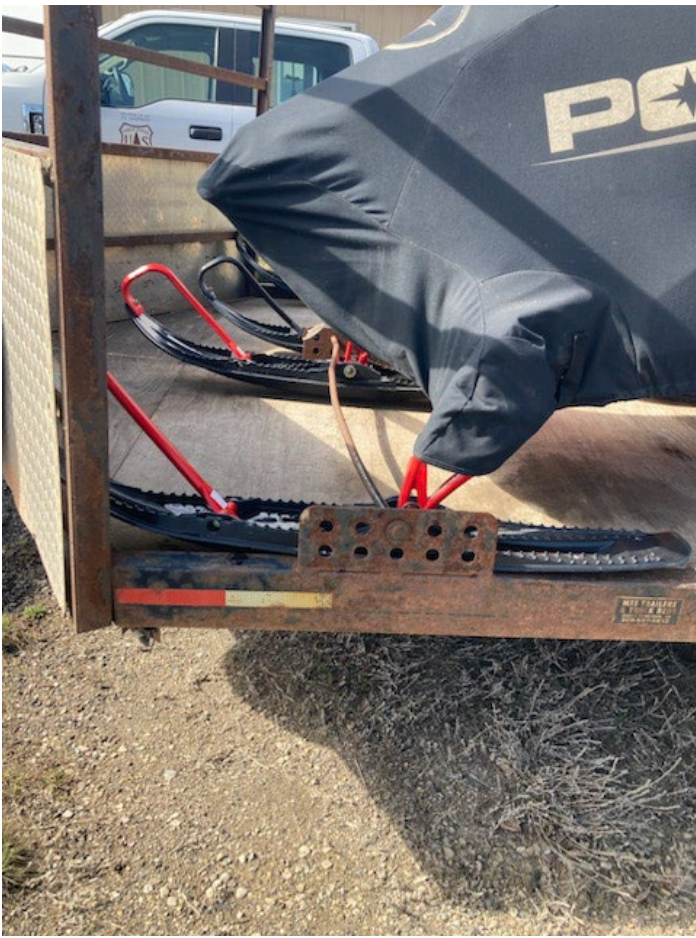
Figure 1. Snowmobile retention system with sliding rods instead of threading system.
