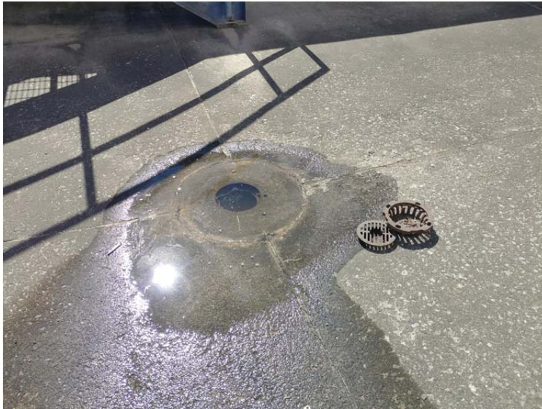
E.4 Secondary Containment Drain Hydrostatic Test
