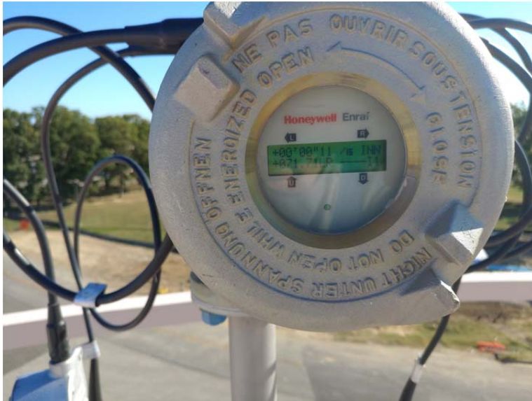
E.61 Roof Nozzle A, 6" Enraf/Vito Stilling Well
