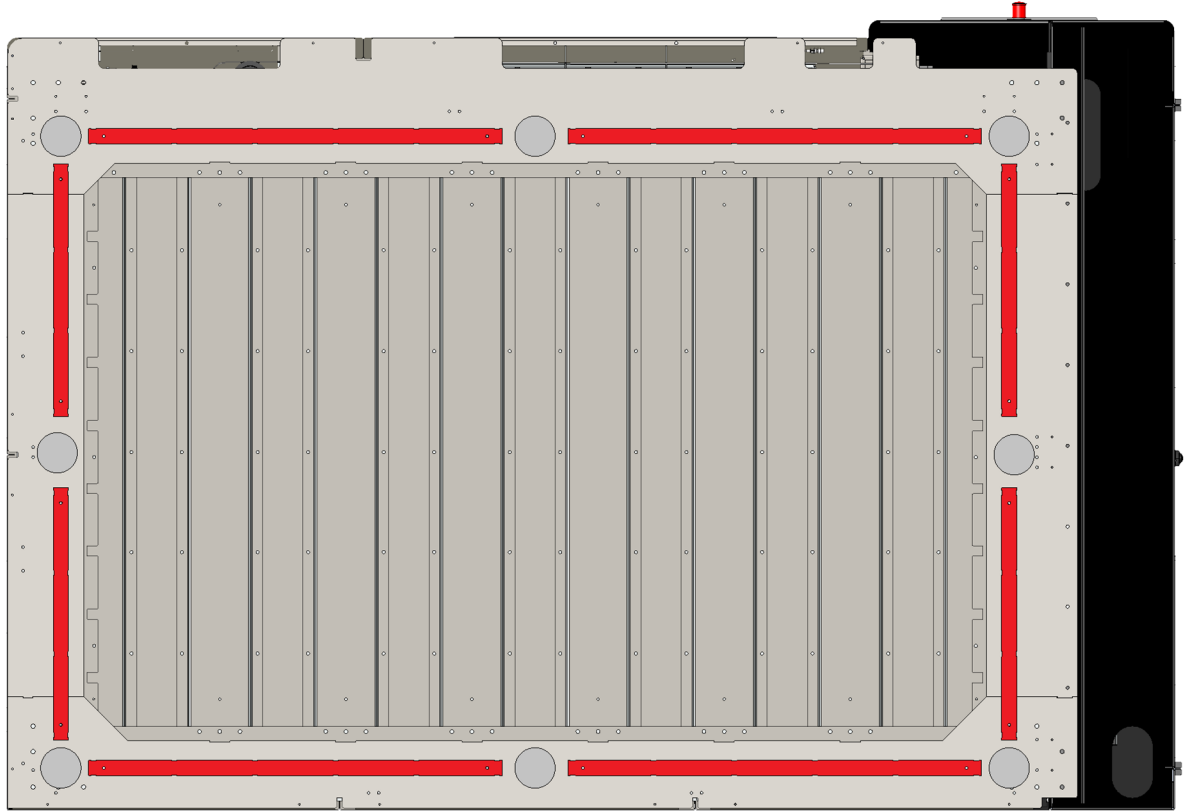
Figure 2 – Lifting should only be completed by areas marked in red.
