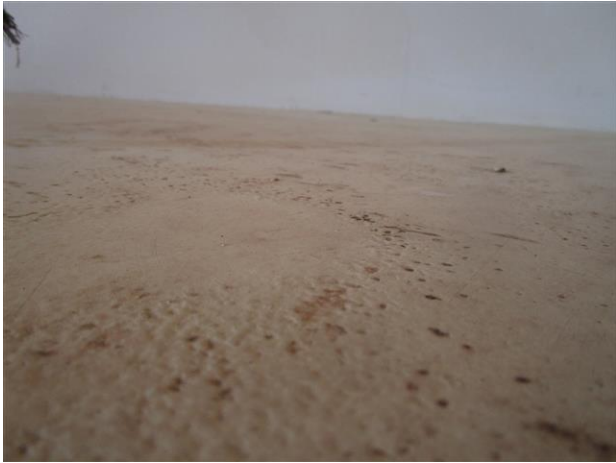
C37: Wide Spread Pitting along the Tank Bottom
