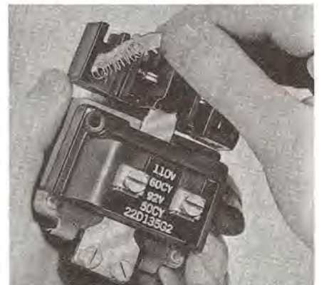
Fig. 3. Method of removing or replacing movable contacts
