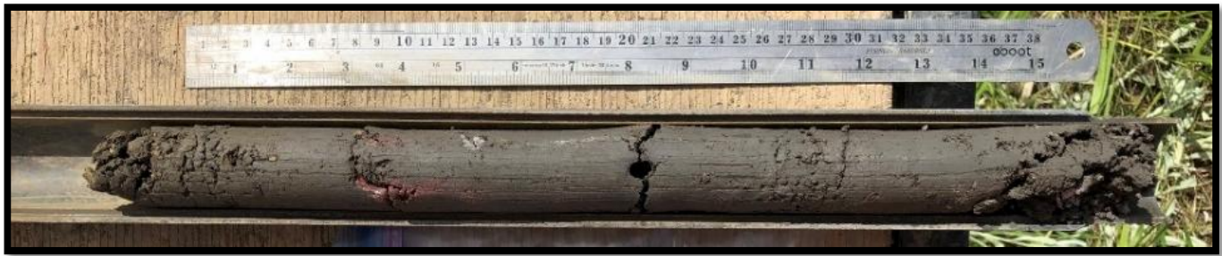
Boring B-4 – Standard Penetration Test Sample – 25.0 to 26.5 feet
