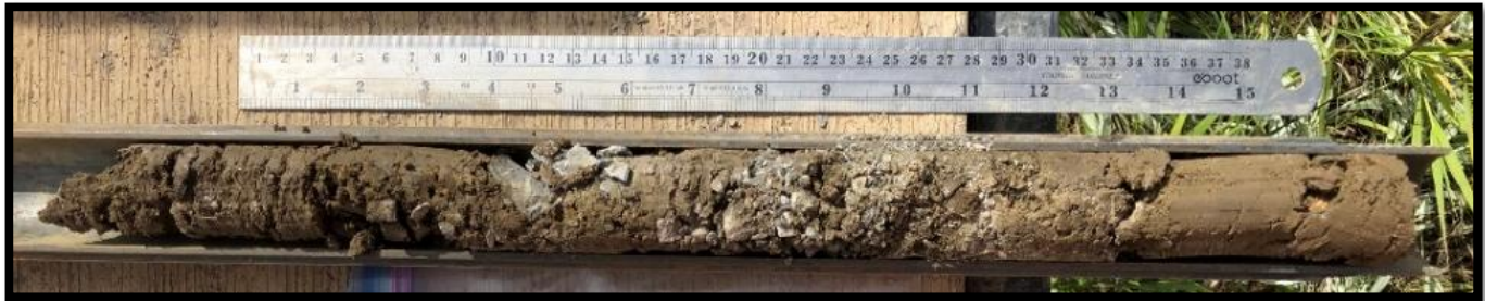
Boring B-4 – Standard Penetration Test Sample – 12.5 to 14.0 feet
