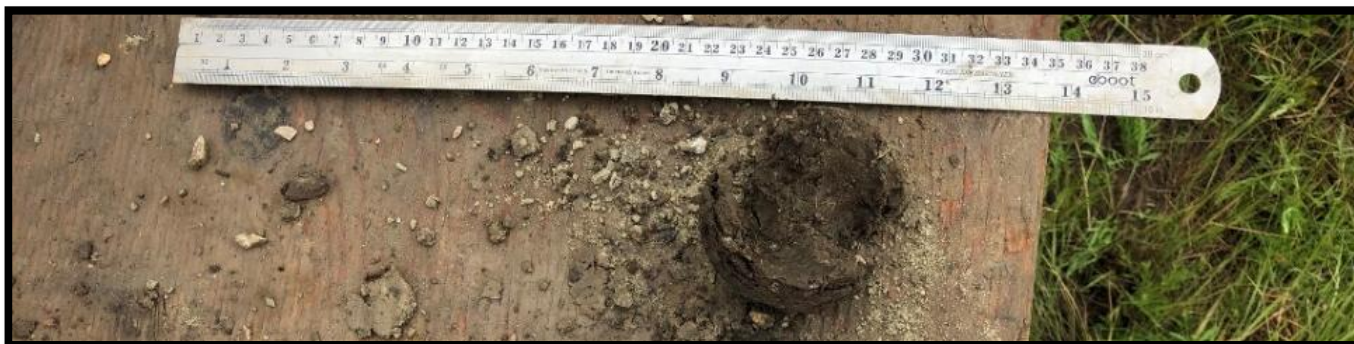
Boring B-2 – Shelby Tube Test Sample – 12.5 to 14.5 feet
