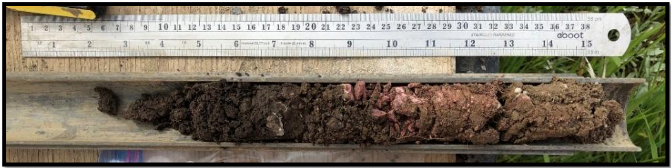
Boring B-4 – Standard Penetration Test Sample – 0.0 to 1.5 feet
