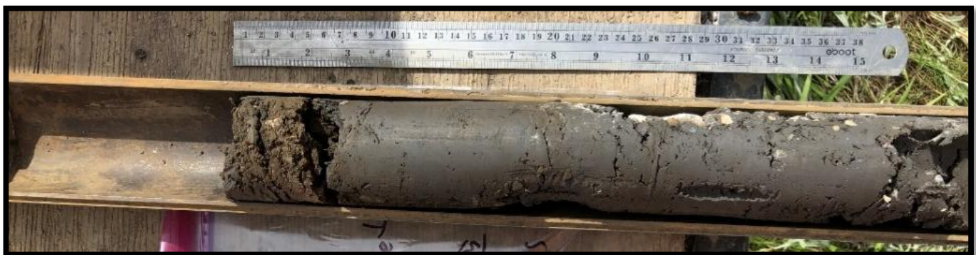
Boring B-4 – Dames and Moore Penetration Test Sample – 20.0 to 21.5 feet
