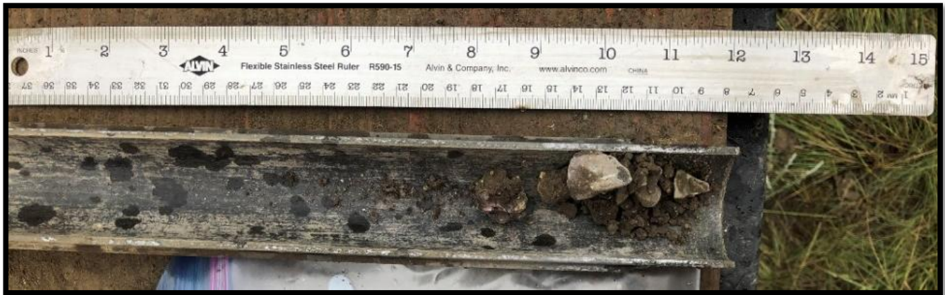
Boring B-6 – Standard Penetration Test Sample – 24.5 to 25.0 feet
