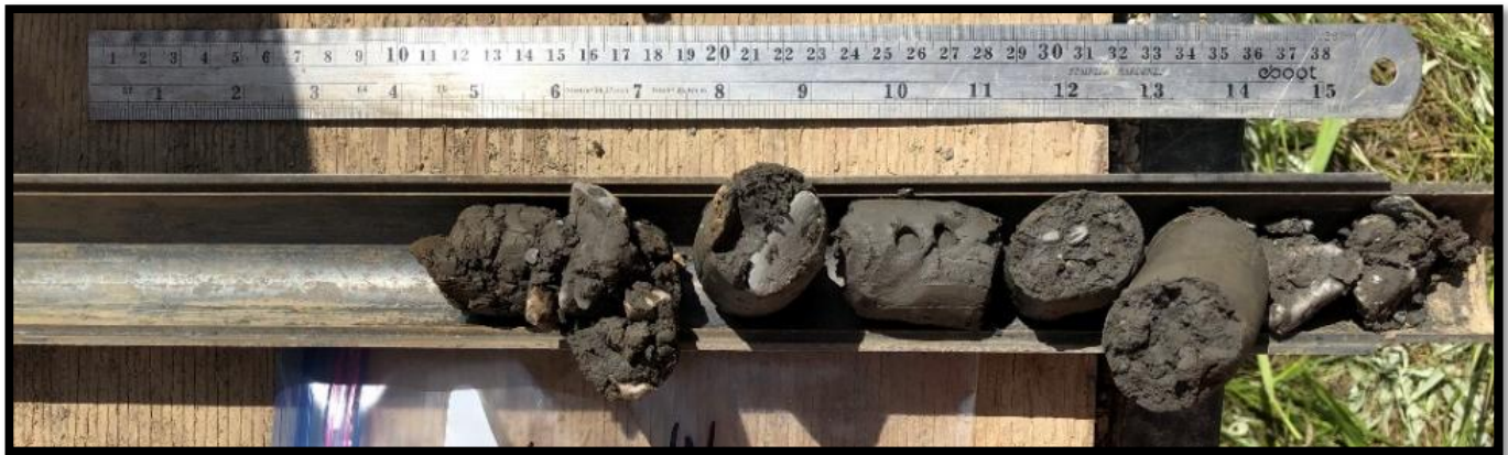
Boring B-4 – Standard Penetration Test Sample – 35.0 to 36.5 feet
