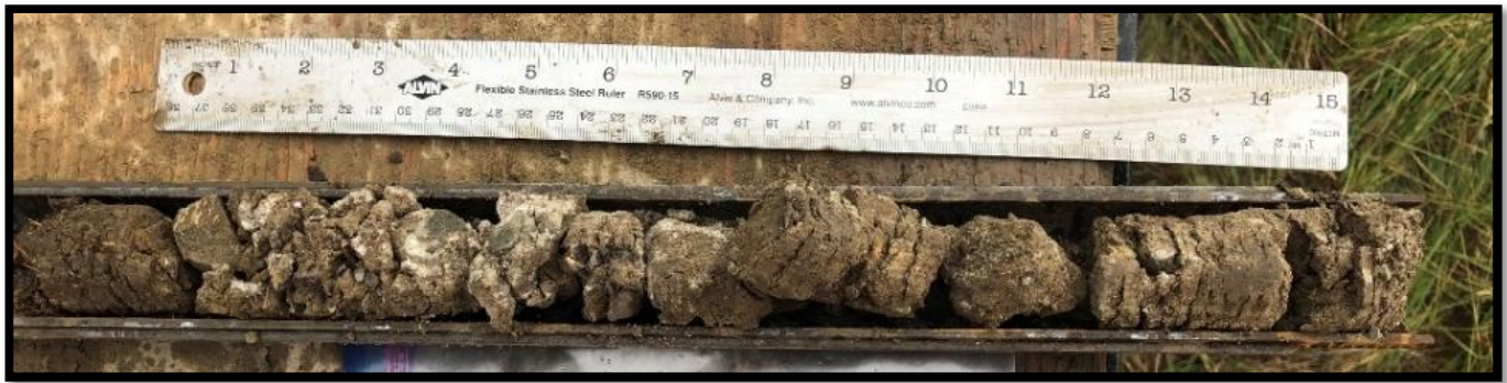
Boring B-3 – Standard Penetration Test Sample – 7.5 to 9.0 feet
