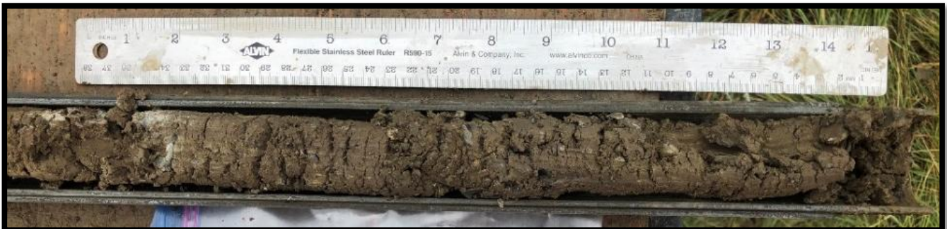
Boring B-6 – Standard Penetration Test Sample – 9.5 to 11.0 feet
