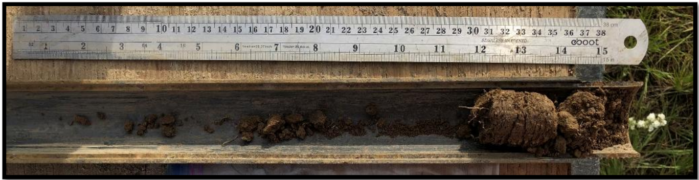
Boring B-1 – Standard Penetration Test Sample – 0.0 to 1.5 feet
