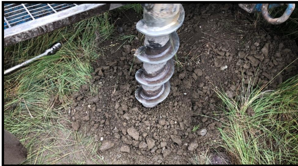
Boring B-6 – Hollow-stem Auger Cuttings – Approximately 12 to 17 feet
