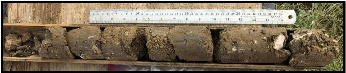
Boring B-1 – Dames and Moore Penetration Test Sample – 12.5 to 14.0 feet
