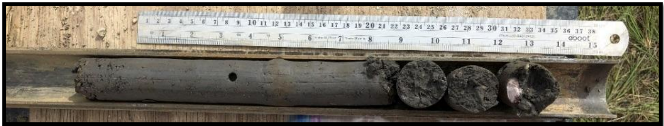
Boring B-1 – Standard Penetration Test Sample – 35.0 to 36.5 feet
