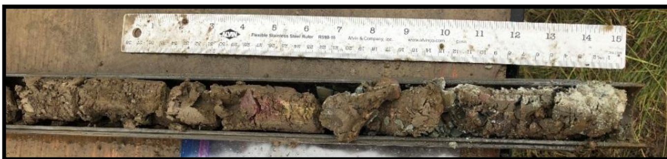
Boring B-3 – Standard Penetration Test Sample – 15.0 to 16.5 feet
