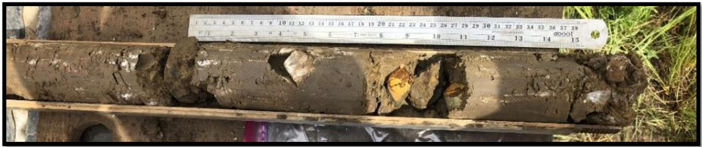
Boring B-2 – Dames and Moore Penetration Test Sample – 20.0 to 21.5 feet
