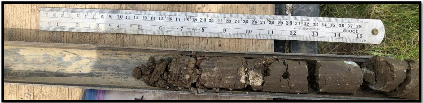
Boring B-8 – Standard Penetration Test Sample – 2.5 to 4.0 feet
