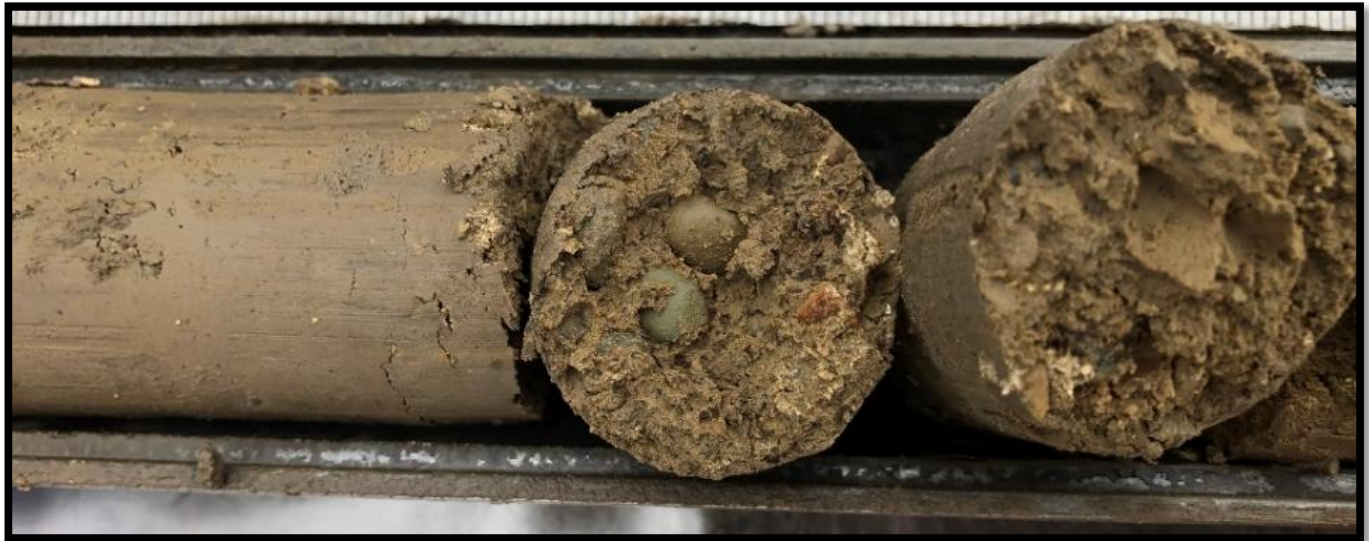
Boring B-5 – Standard Penetration Test Sample – 13.5 to 13.8 feet
