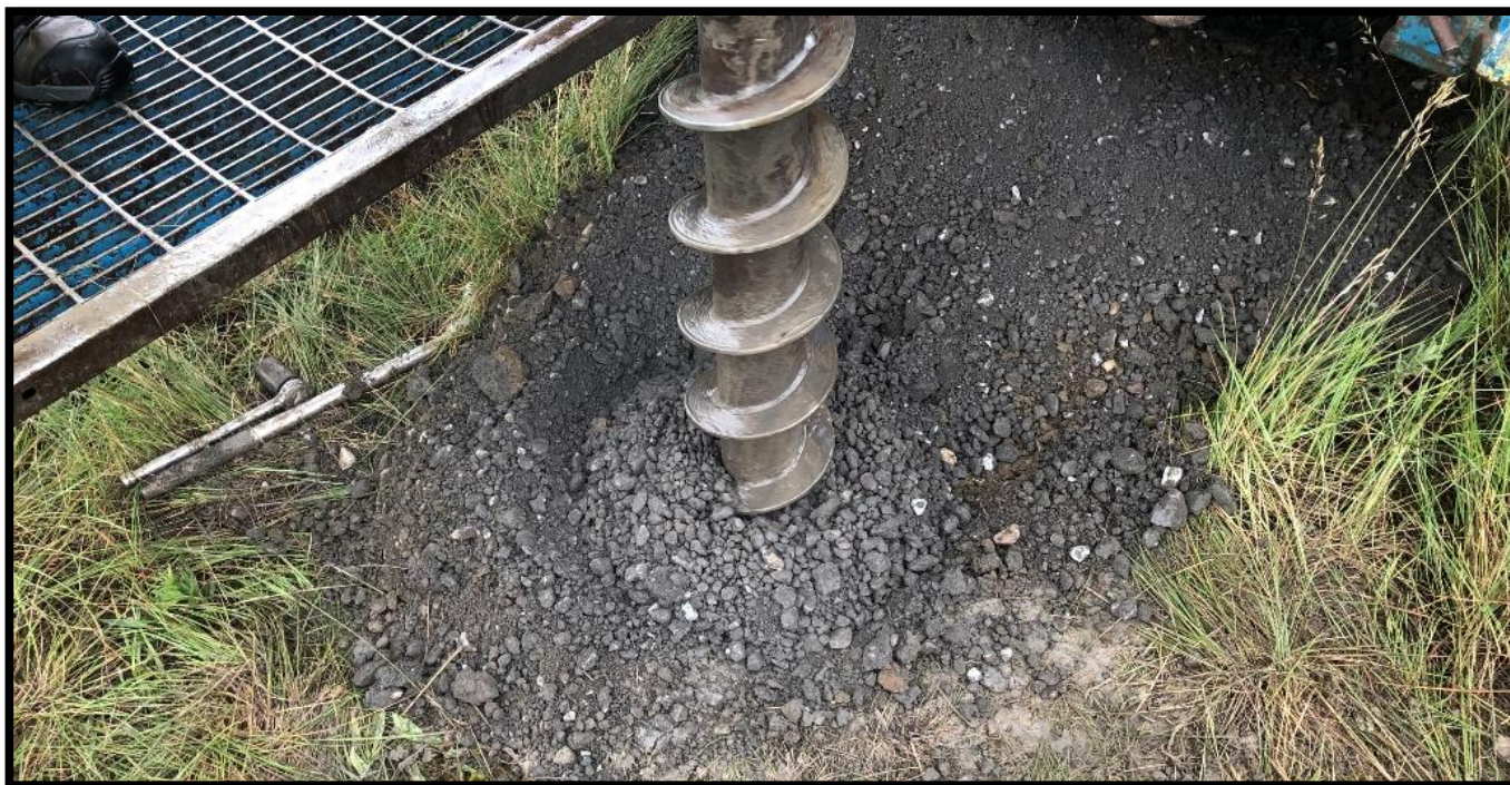
Boring B-3 – Hollow-stem Auger Cuttings – Approximately 25 to 30 feet
