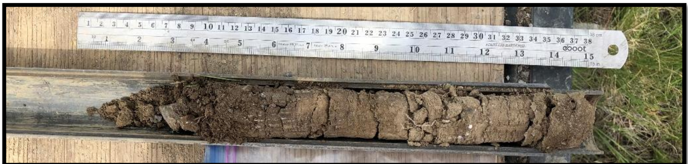
Boring B-8 – Standard Penetration Test Sample – 0.0 to 1.5 feet
