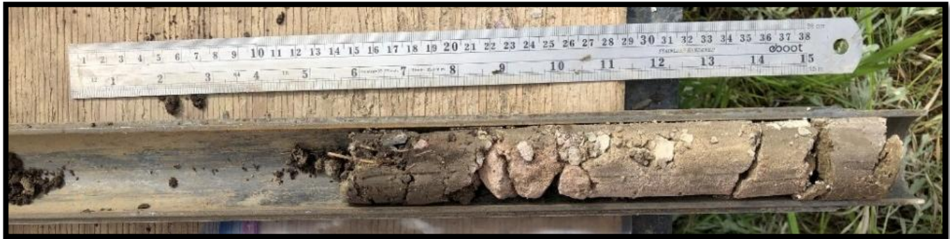
Boring B-4 – Standard Penetration Test Sample – 2.5 to 4.0 feet
