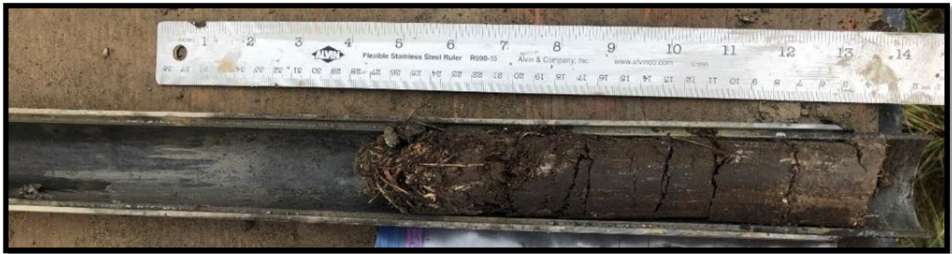
Boring B-6 – Standard Penetration Test Sample – 0.0 to 1.5 feet
