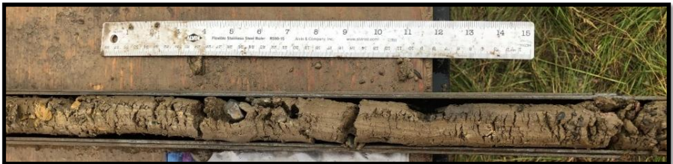
Boring B-3 – Standard Penetration Test Sample – 12.5 to 14.0 feet
