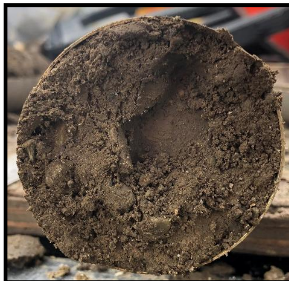
Boring B-2 – Dames and Moore Penetration Test Sample – 9.0 feet
