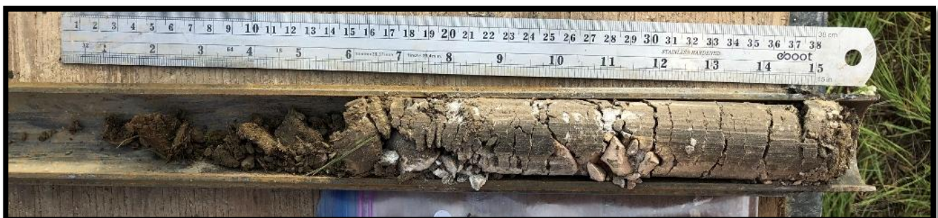
Boring B-1 – Standard Penetration Test Sample – 7.5 to 9.0 feet
