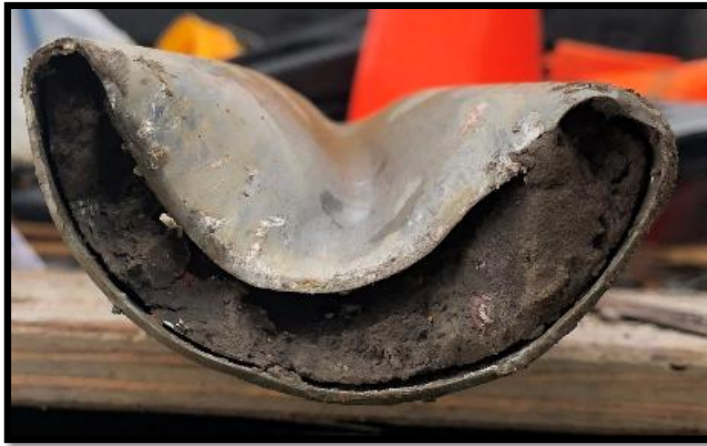
Boring B-5 – Shelby Tube Test Sample – 30.0 to 32.0 feet
