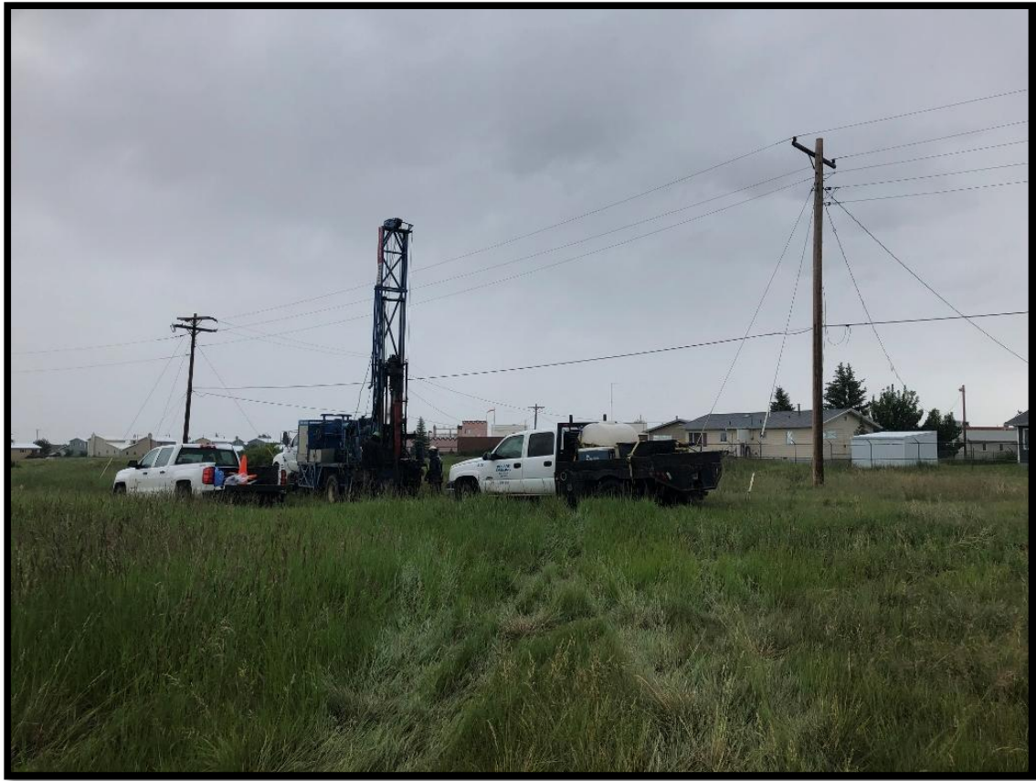
Drilling Boring B-5 – View Northeast – Mobile B-59 Truck-Mounted Drill Rig
