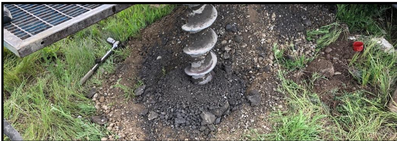
Boring B-1 – Hollow-stem Auger Cuttings – Approximately 23 to 28 feet
