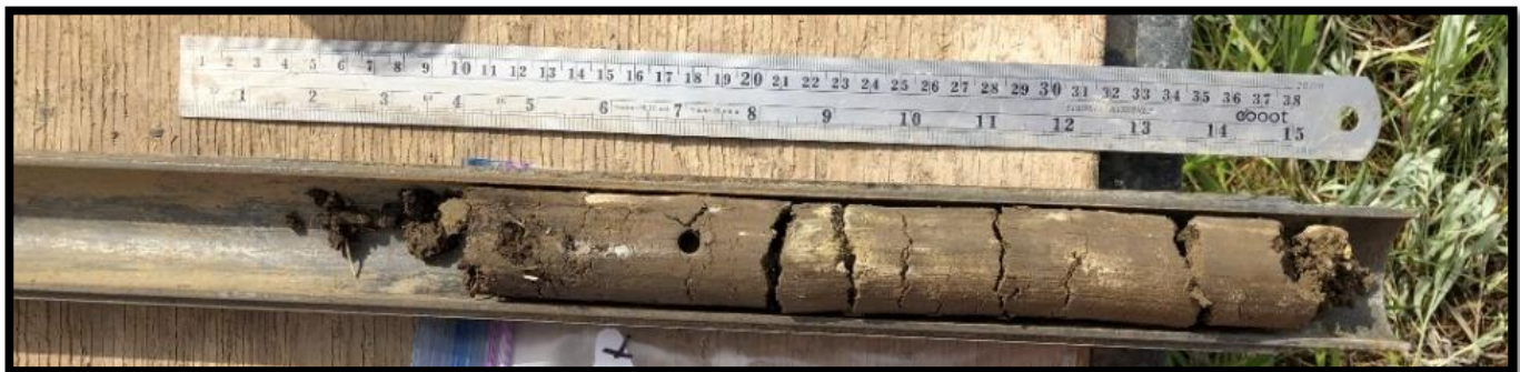
Boring B-4 – Standard Penetration Test Sample – 7.5 to 9.0 feet
