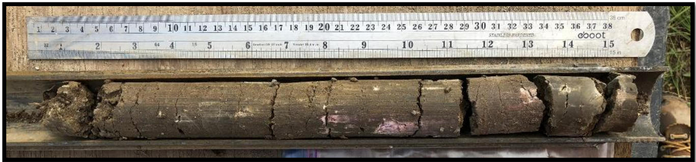
Boring B-1 – Standard Penetration Test Sample – 10.0 to 11.5 feet
