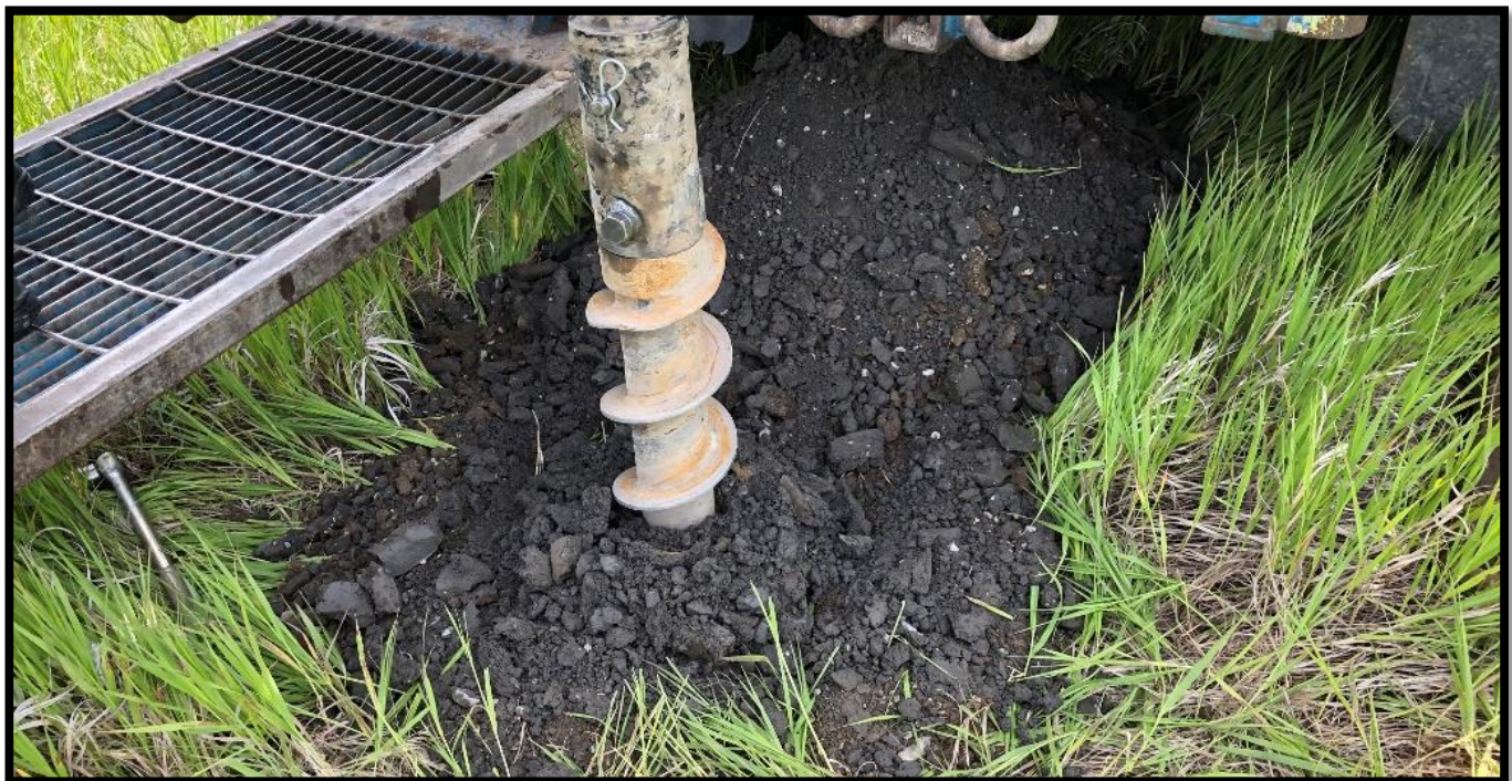
Boring B-4 – Hollow-stem Auger Cuttings – Approximately 25 to 33 feet
