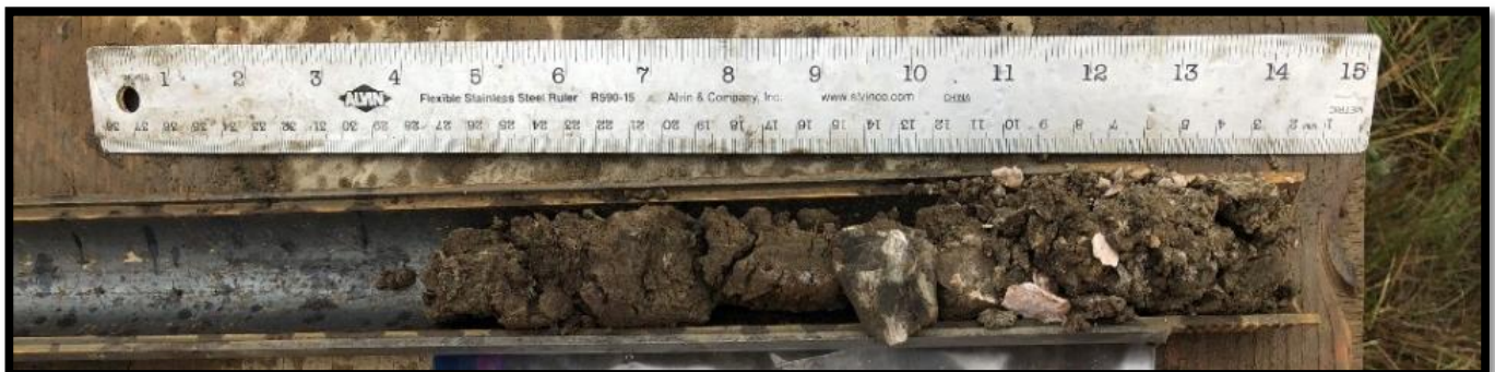
Boring B-3 – Standard Penetration Test Sample – 5.0 to 6.5 feet
