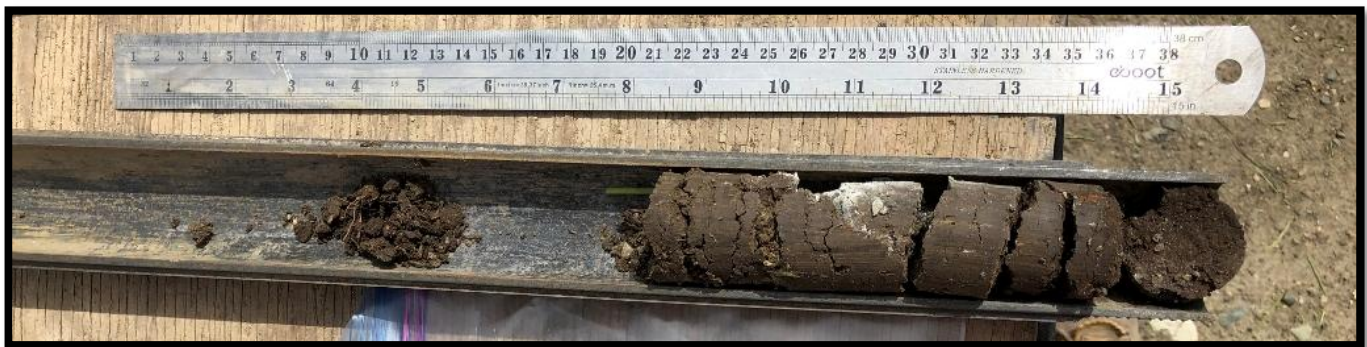
Boring B-7 – Standard Penetration Test Sample – 2.5 to 4.0 feet
