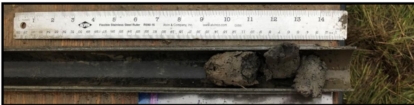
Boring B-3 – Standard Penetration Test Sample – 20.0 to 21.5 feet
