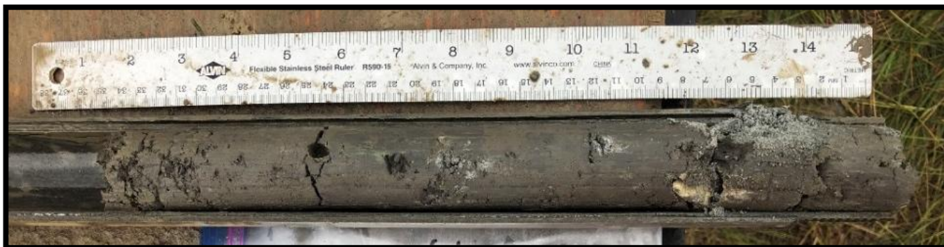
Boring B-3 – Standard Penetration Test Sample – 30.0 to 31.5 feet
