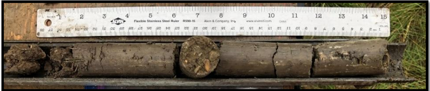
Boring B-3 – Standard Penetration Test Sample – 10.0 to 11.5 feet
