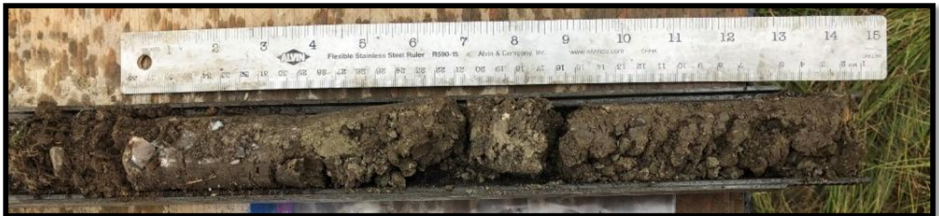
Boring B-3 – Standard Penetration Test Sample – 2.5 to 4.0 feet
