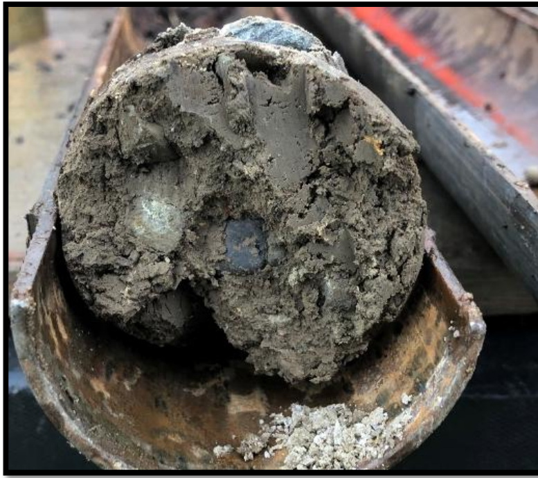
Boring B-5 – Dames and Moore Penetration Test Sample – 6.5 feet
