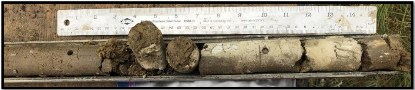
Boring B-6 – Standard Penetration Test Sample – 15.0 to 16.5 feet
