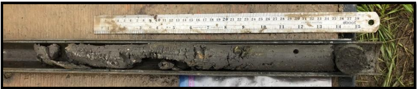
Boring B-5 – Standard Penetration Test Sample – 32.0 to 33.5 feet
