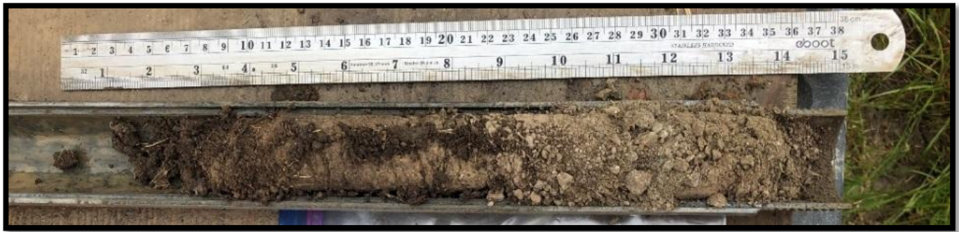
Boring B-2 – Standard Penetration Test Sample – 0.0 to 1.5 feet
