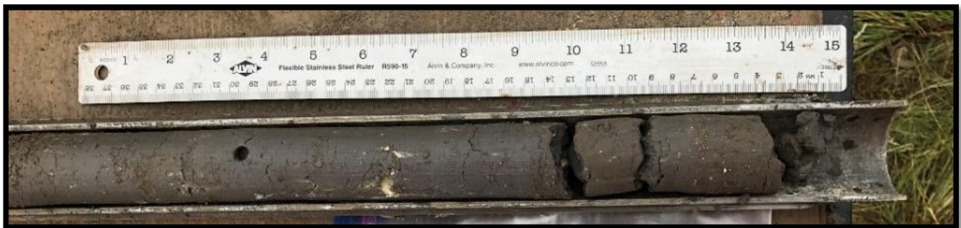
Boring B-6 – Standard Penetration Test Sample – 30.0 to 31.5 feet
