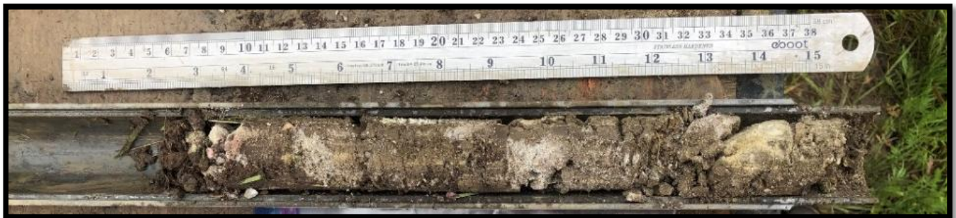
Boring B-2 – Standard Penetration Test Sample – 5.0 to 6.5 feet
