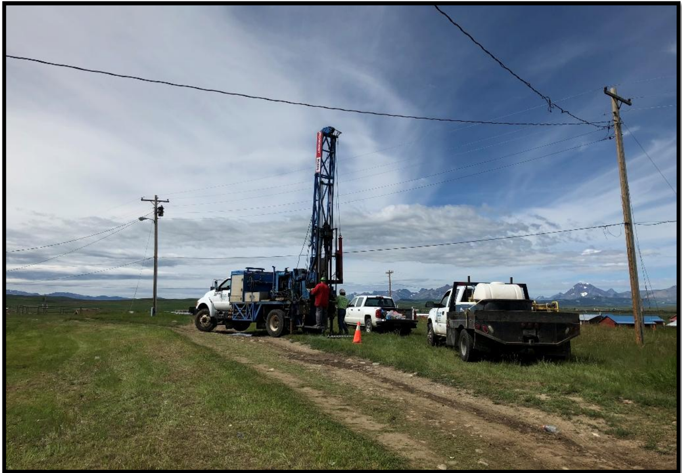
Drilling Boring B-8 – View Southwest – Mobile B-59 Truck-Mounted Drill Rig
