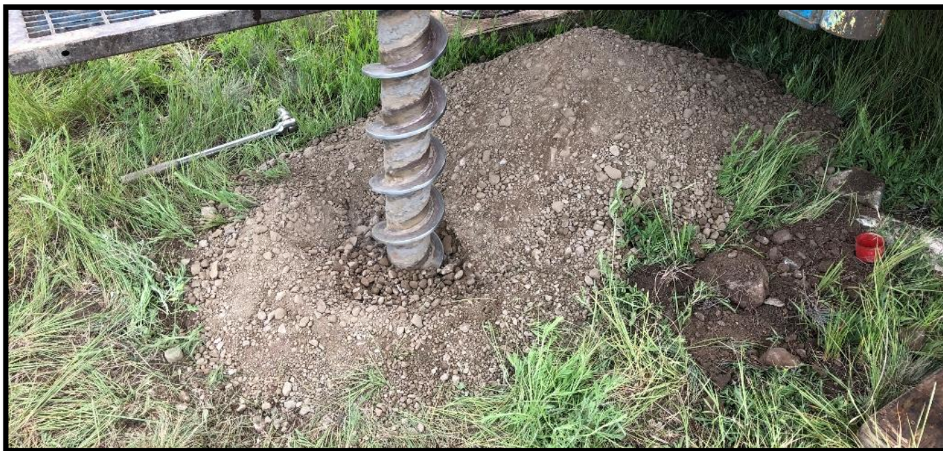
Boring B-1 – Hollow-stem Auger Cuttings – Approximately 10 to 18 feet
