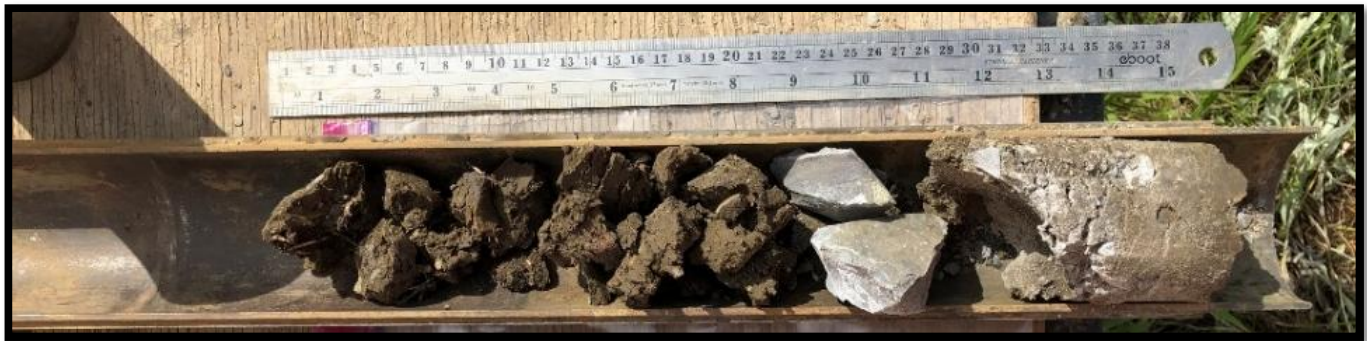
Boring B-4 – Dames and Moore Penetration Test Sample – 10.0 to 11.5 feet
