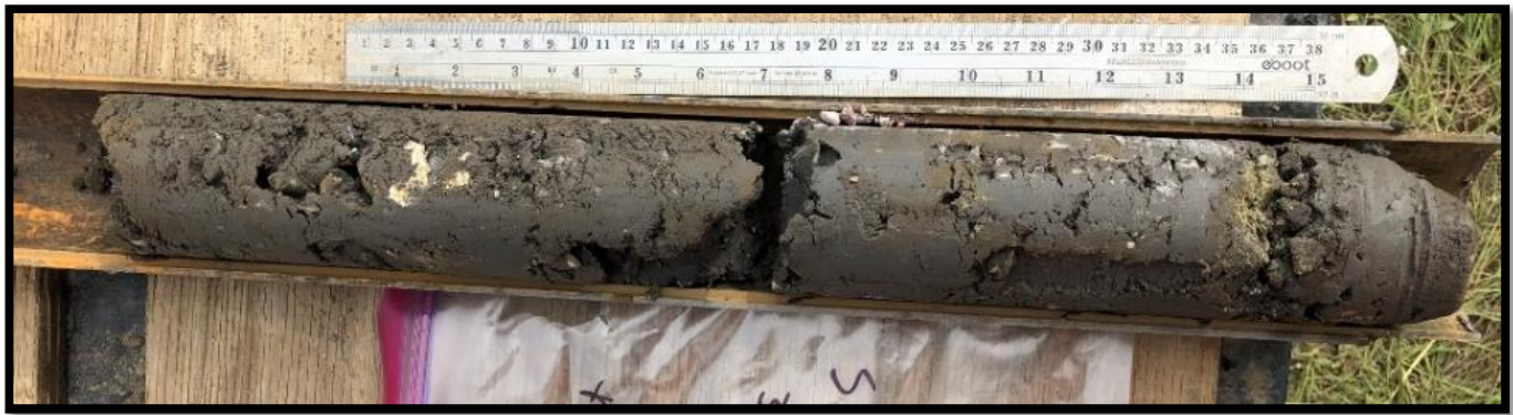
Boring B-1 – Dames and Moore Penetration Test Sample – 30.0 to 31.5 feet
