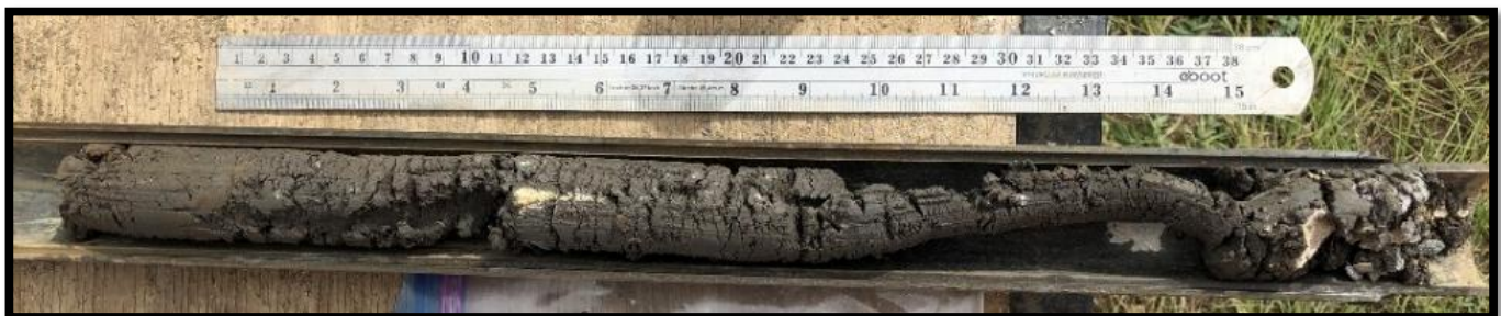
Boring B-1 – Standard Penetration Test Sample – 40.0 to 41.5 feet
