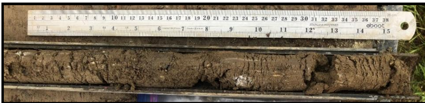
Boring B-2 – Standard Penetration Test Sample – 10.0 to 11.5 feet
