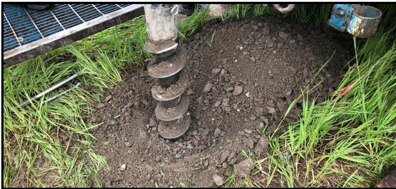
Boring B-5 – Hollow-stem Auger Cuttings – Approximately 10 to 16 feet
