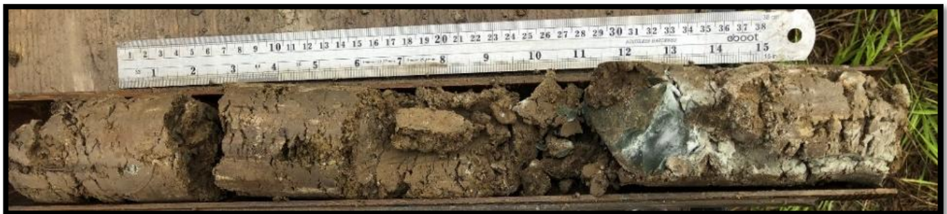
Boring B-5 – Dames and Moore Penetration Test Sample – 15.0 to 16.5 feet
