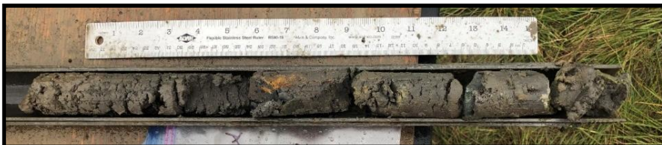
Boring B-3 – Standard Penetration Test Sample – 25.0 to 26.5 feet
