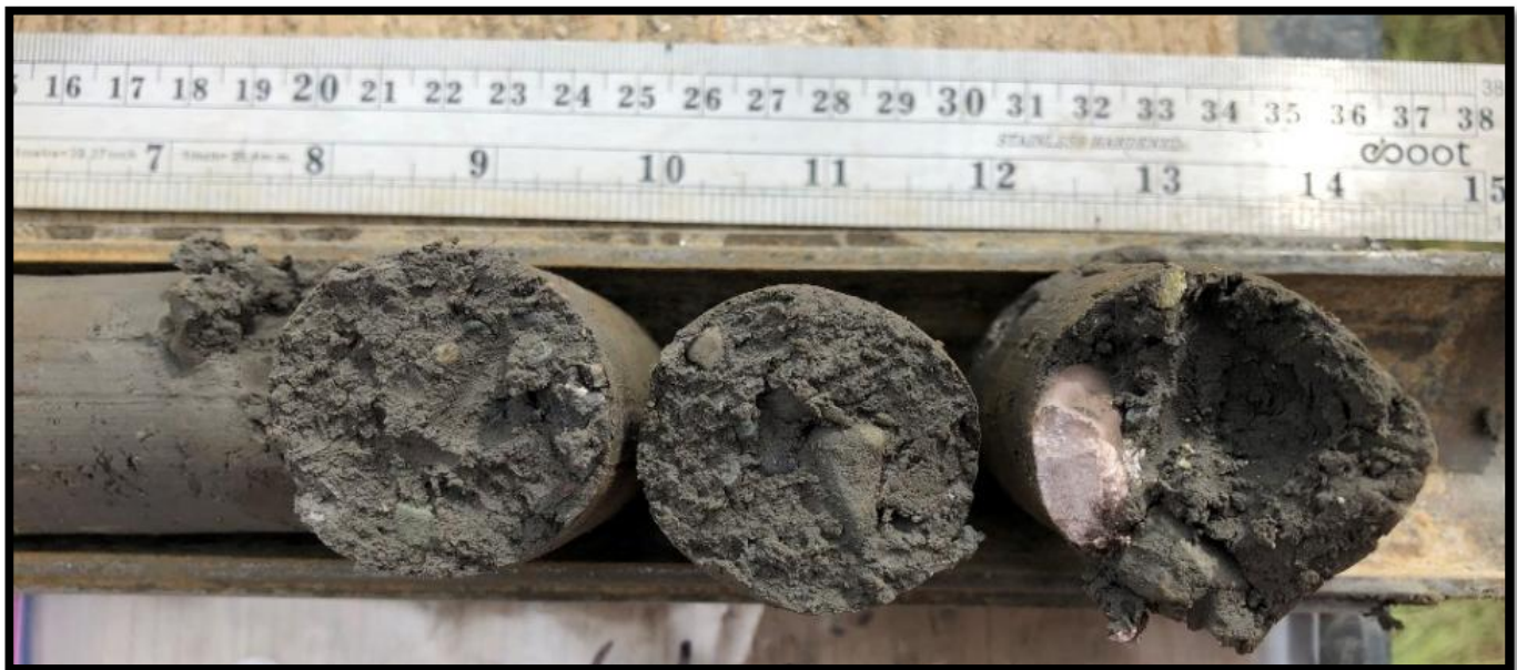
Boring B-1 – Standard Penetration Test Sample – 36.0 to 36.5 feet
