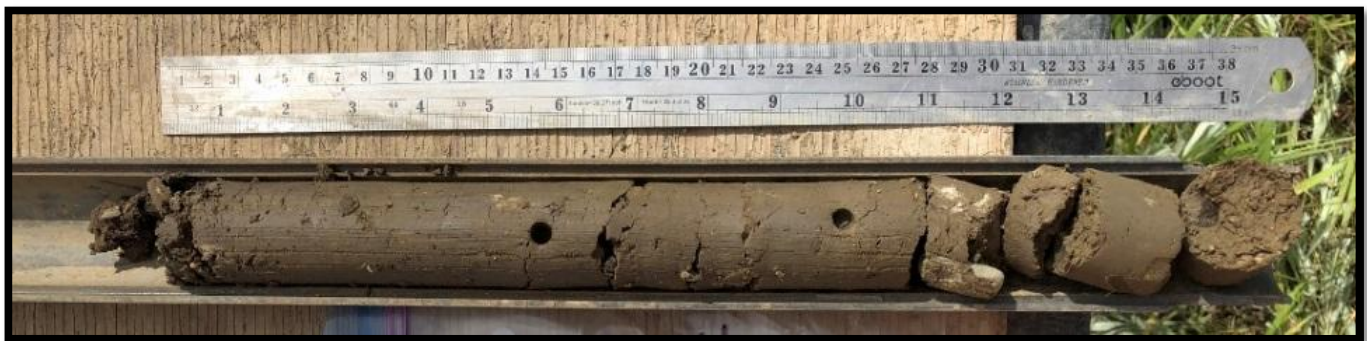
Boring B-4 – Standard Penetration Test Sample – 15.0 to 16.5 feet
