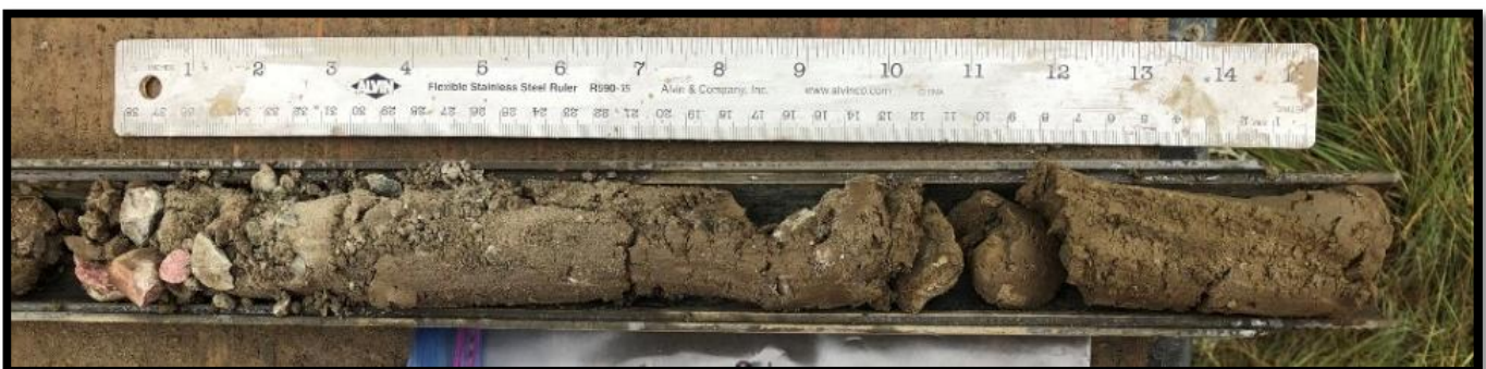
Boring B-6 – Standard Penetration Test Sample – 12.5 to 14.0 feet
