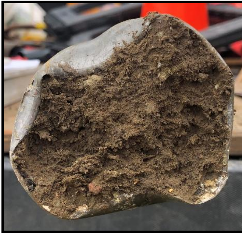
Boring B-6 – Shelby Tube Test Sample – 7.5 to 9.5 feet
