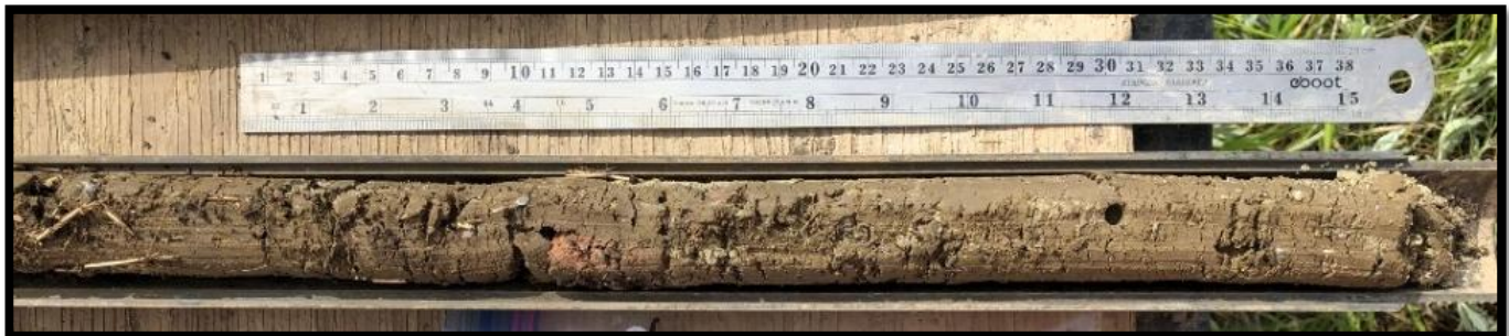
Boring B-4 – Standard Penetration Test Sample – 5.0 to 6.5 feet
