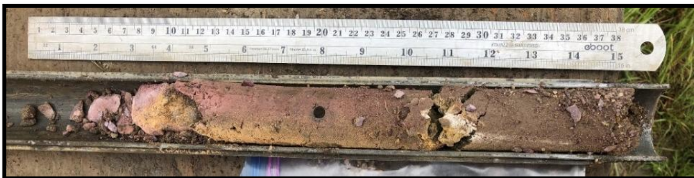
Boring B-2 – Standard Penetration Test Sample – 15.5 to 16.0 feet
