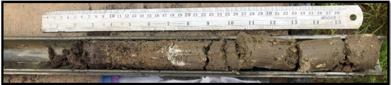
Boring B-2 – Standard Penetration Test Sample – 2.5 to 4.0 feet
