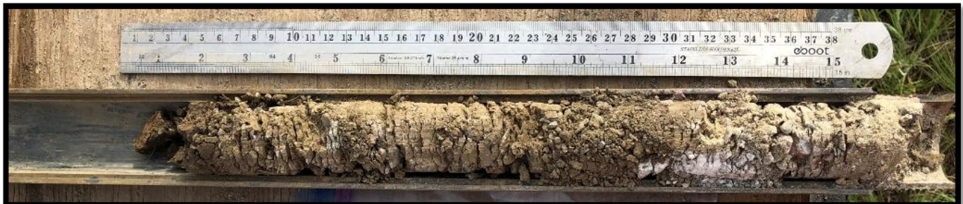
Boring B-1 – Standard Penetration Test Sample – 5.0 to 6.5 feet
