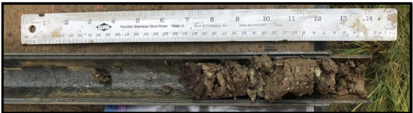
Boring B-6 – Standard Penetration Test Sample – 5.0 to 6.5 feet
