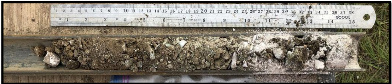
Boring B-1 – Standard Penetration Test Sample – 20.0 to 21.5 feet
