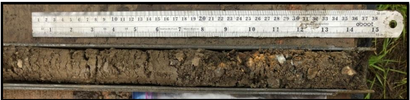
Boring B-5 – Standard Penetration Test Sample – 10.0 to 11.5 feet
