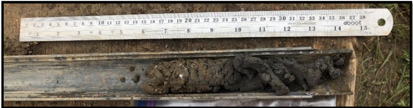
Boring B-2 – Standard Penetration Test Sample – 25.0 to 26.5 feet
