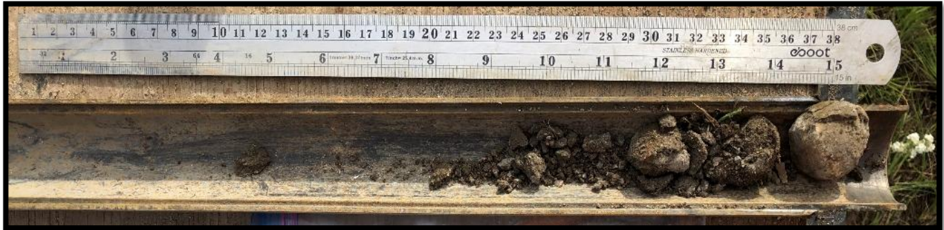
Boring B-1 – Standard Penetration Test Sample – 2.5 to 4.0 feet
