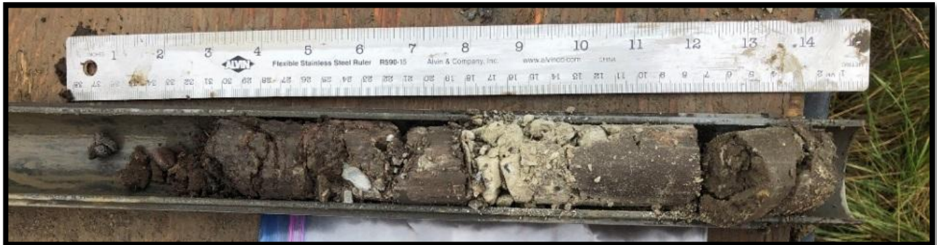
Boring B-6 – Standard Penetration Test Sample – 2.5 to 4.0 feet
