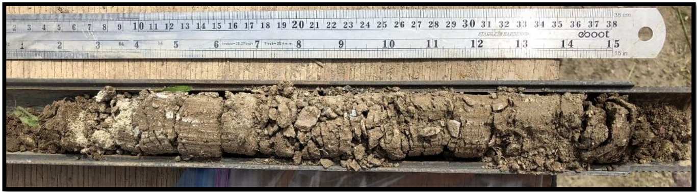
Boring B-7 – Standard Penetration Test Sample – 0.0 to 1.5 feet
