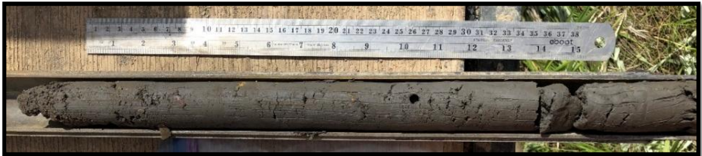
Boring B-4 – Standard Penetration Test Sample – 30.0 to 31.5 feet
