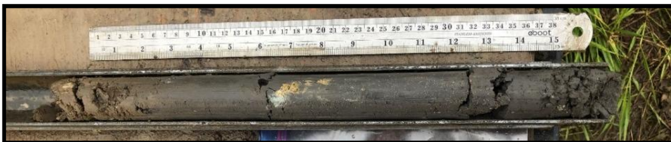
Boring B-5 – Standard Penetration Test Sample – 20.0 to 21.5 feet
