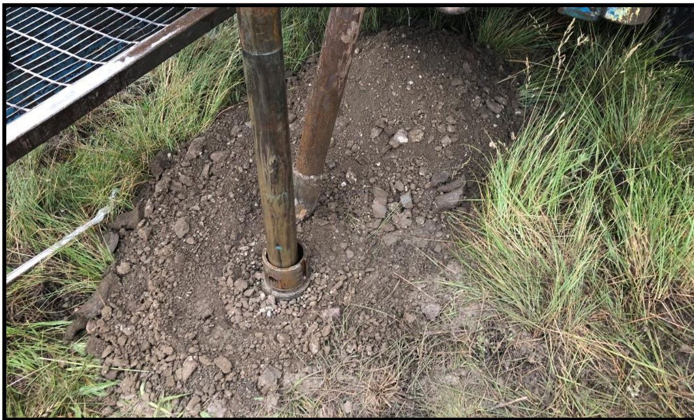
Boring B-3 – Hollow-stem Auger Cuttings – Approximately 5 to 10 feet
