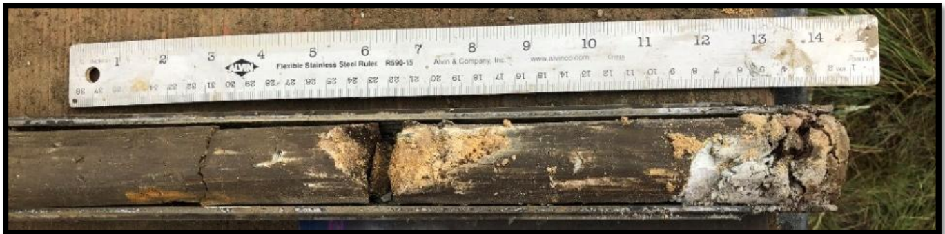
Boring B-6 – Standard Penetration Test Sample – 20.0 to 21.5 feet
