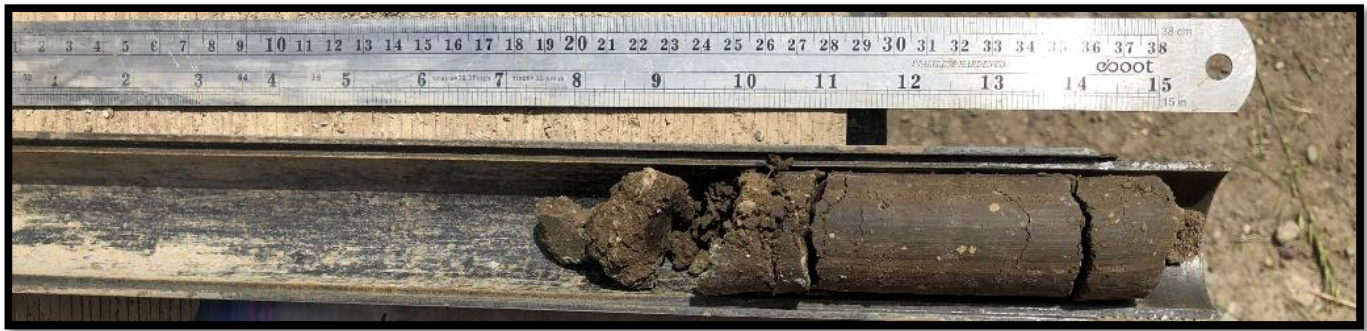
Boring B-7 – Standard Penetration Test Sample – 10.0 to 11.5 feet
