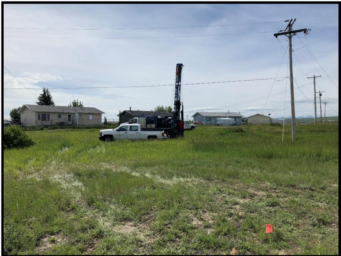
Drilling Boring B-4 – View Southeast – Mobile B-59 Truck-Mounted Drill Rig
