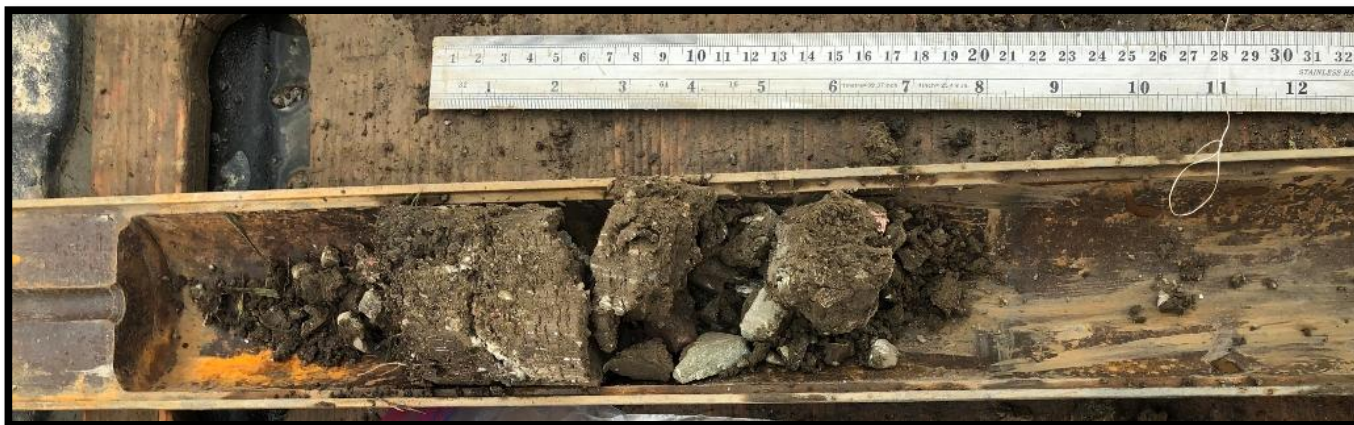
Boring B-2 – Dames and Moore Penetration Test Sample – 7.5 to 8.0 feet
