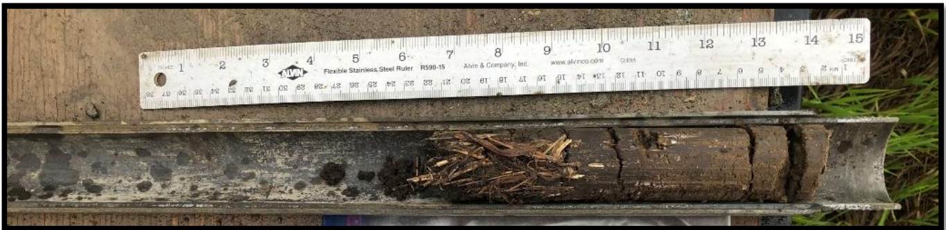
Boring B-5 – Standard Penetration Test Sample – 0.0 to 1.5 feet
