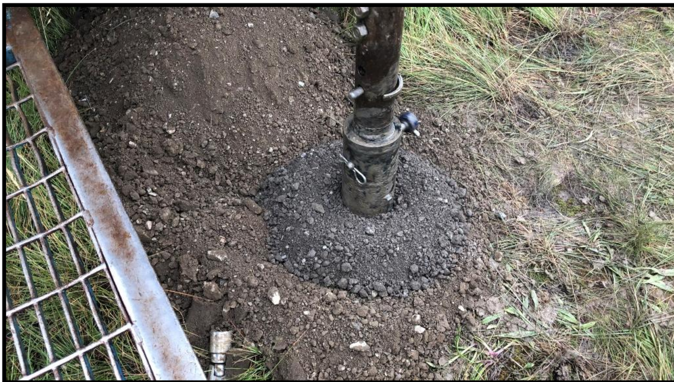
Boring B-3 – Hollow-stem Auger Cuttings – Approximately 17 to 19 feet
