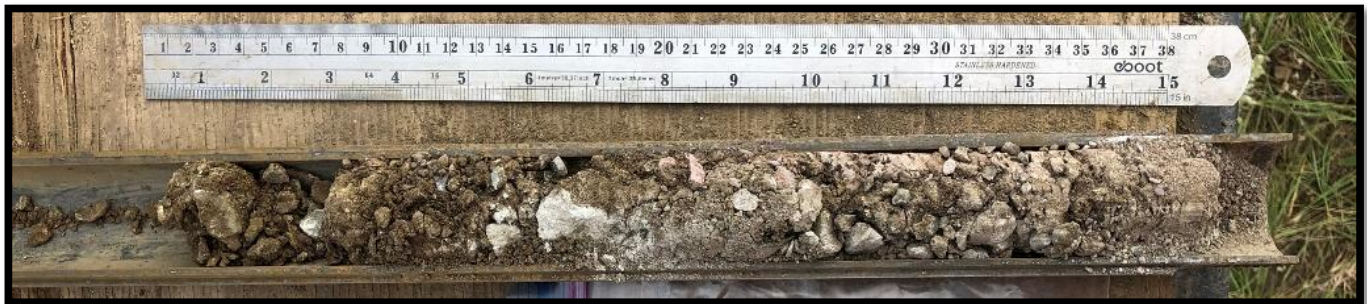
Boring B-1 – Standard Penetration Test Sample – 15.0 to 16.5 feet
