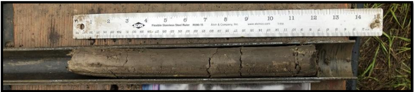
Boring B-5 – Standard Penetration Test Sample – 7.5 to 9.0 feet
