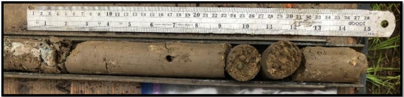
Boring B-5 – Standard Penetration Test Sample – 12.5 to 14.0 feet
