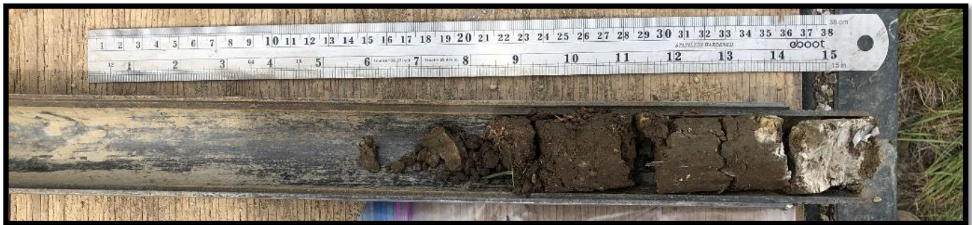
Boring B-8 – Standard Penetration Test Sample – 7.5 to 9.0 feet
