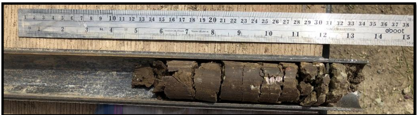
Boring B-7 – Standard Penetration Test Sample – 7.5 to 9.0 feet
