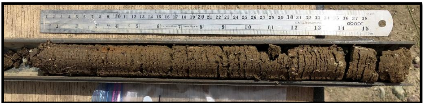
Boring B-7 – Standard Penetration Test Sample – 5.0 to 6.5 feet
