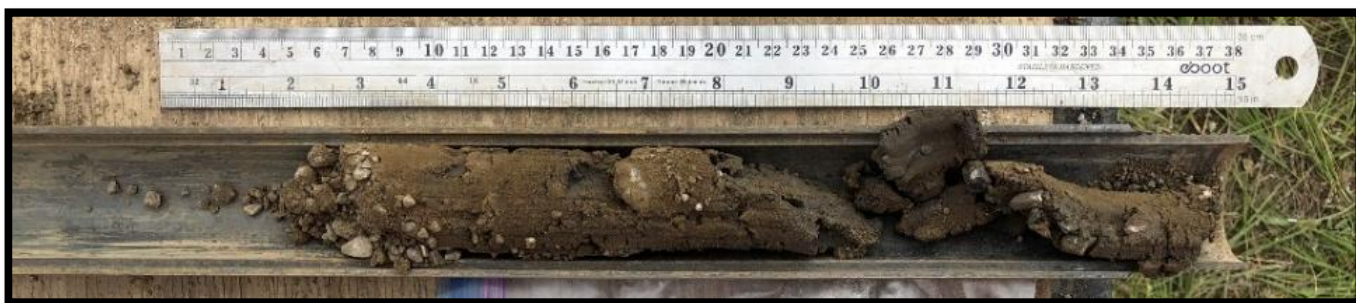
Boring B-1 – Standard Penetration Test Sample – 25.0 to 26.5 feet
