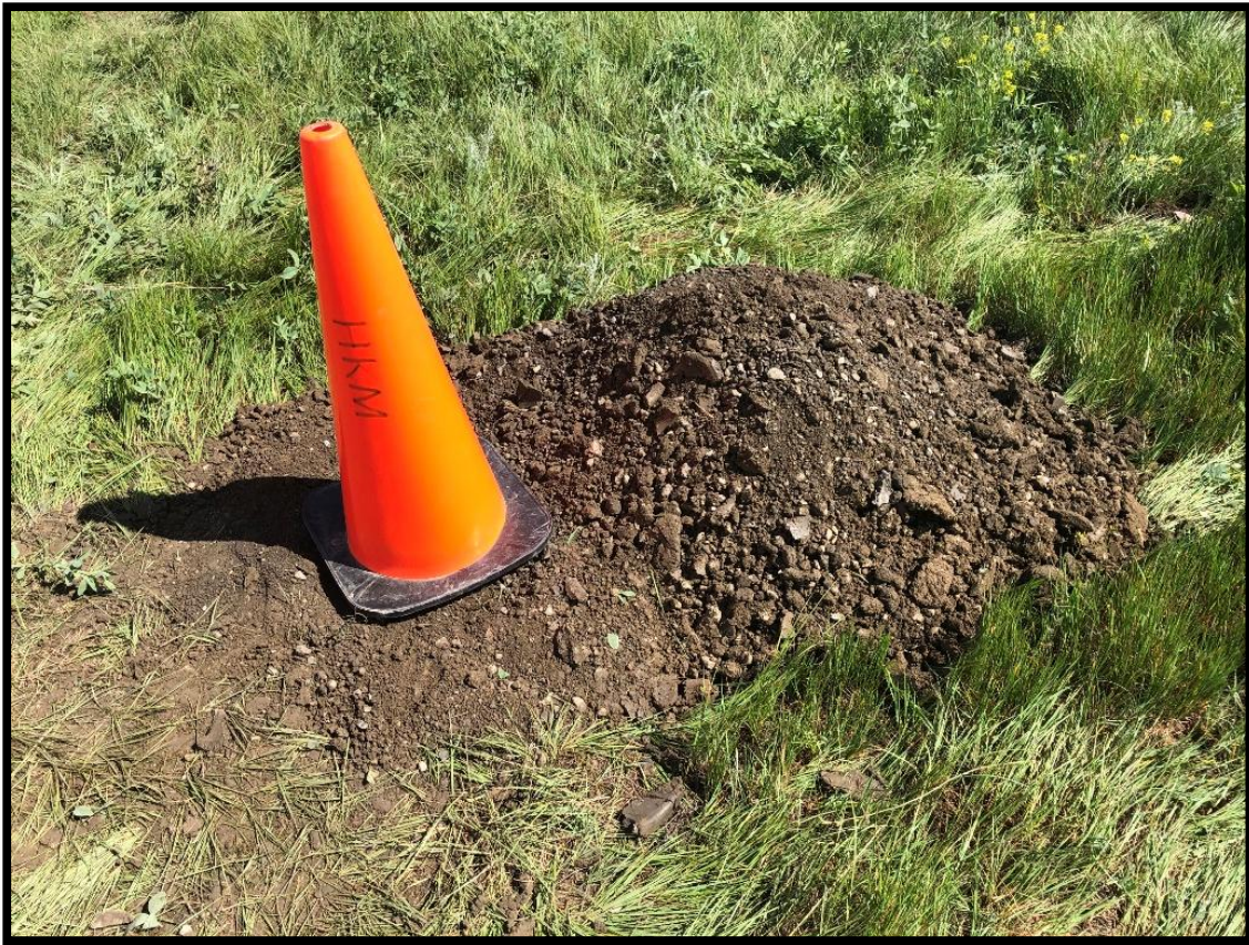
Boring B-2 – Hollow-stem Auger Cuttings – Approximately 20 to 30 feet
