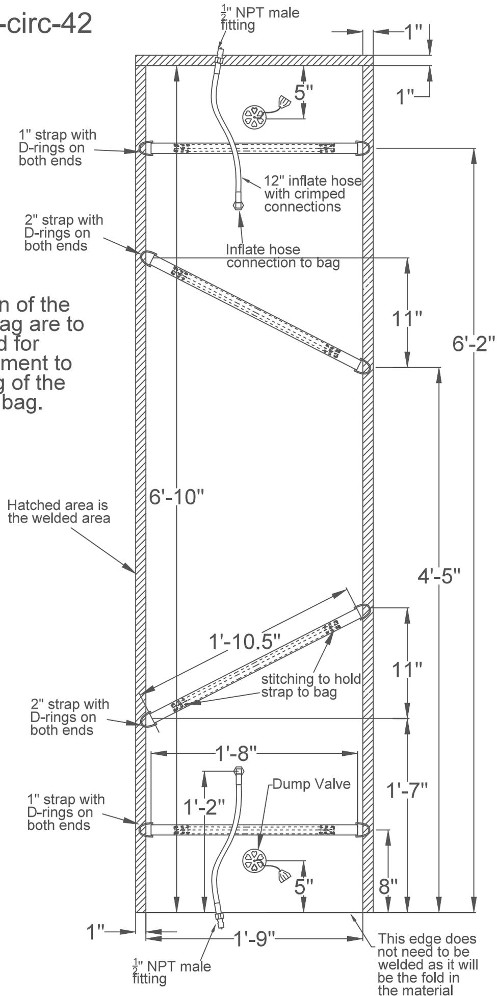
The connection of the straps to the bag are to be multilayered for extra reinforcement to prevent tearing of the strap from the bag.
