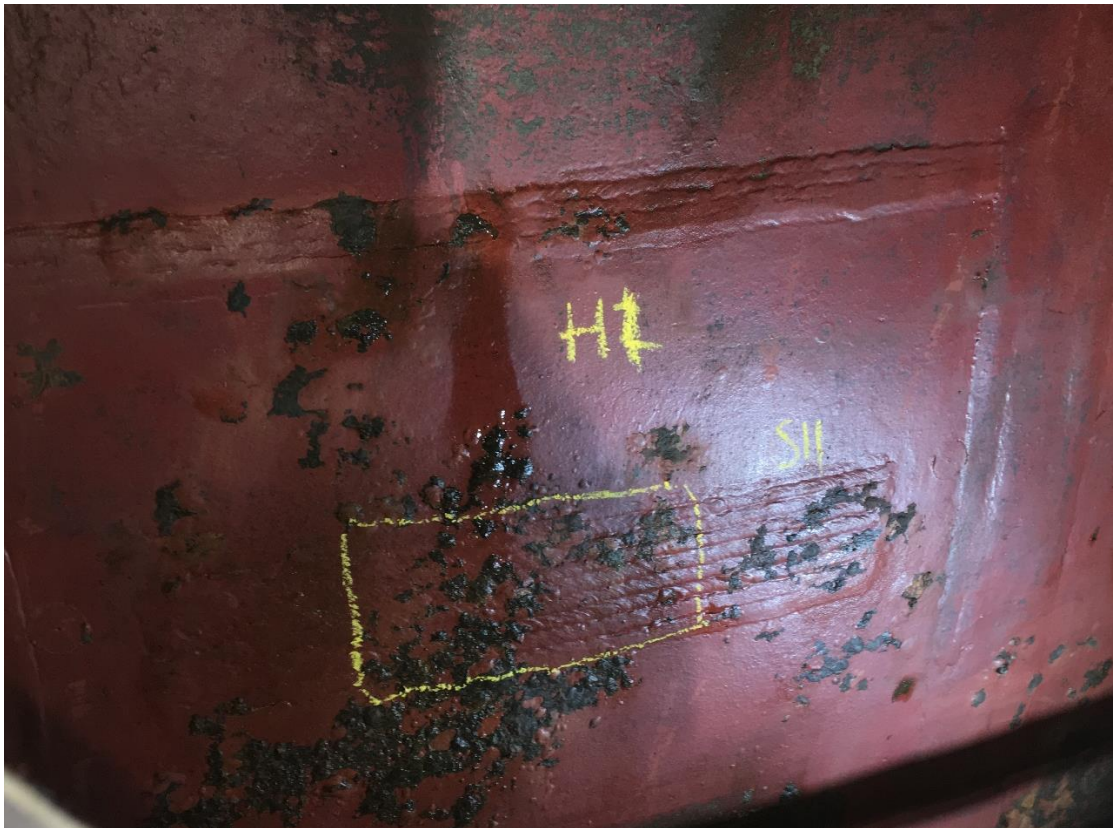
Figure 2.3: Example cleaned surfaces on Valve 4 upstream welds H1 and S11.
