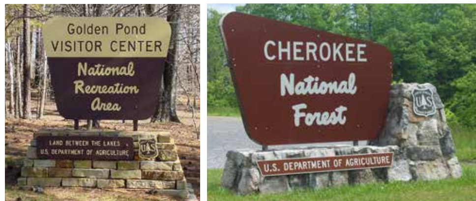
Figure 8-2—Solid bases outside of clear zone.
