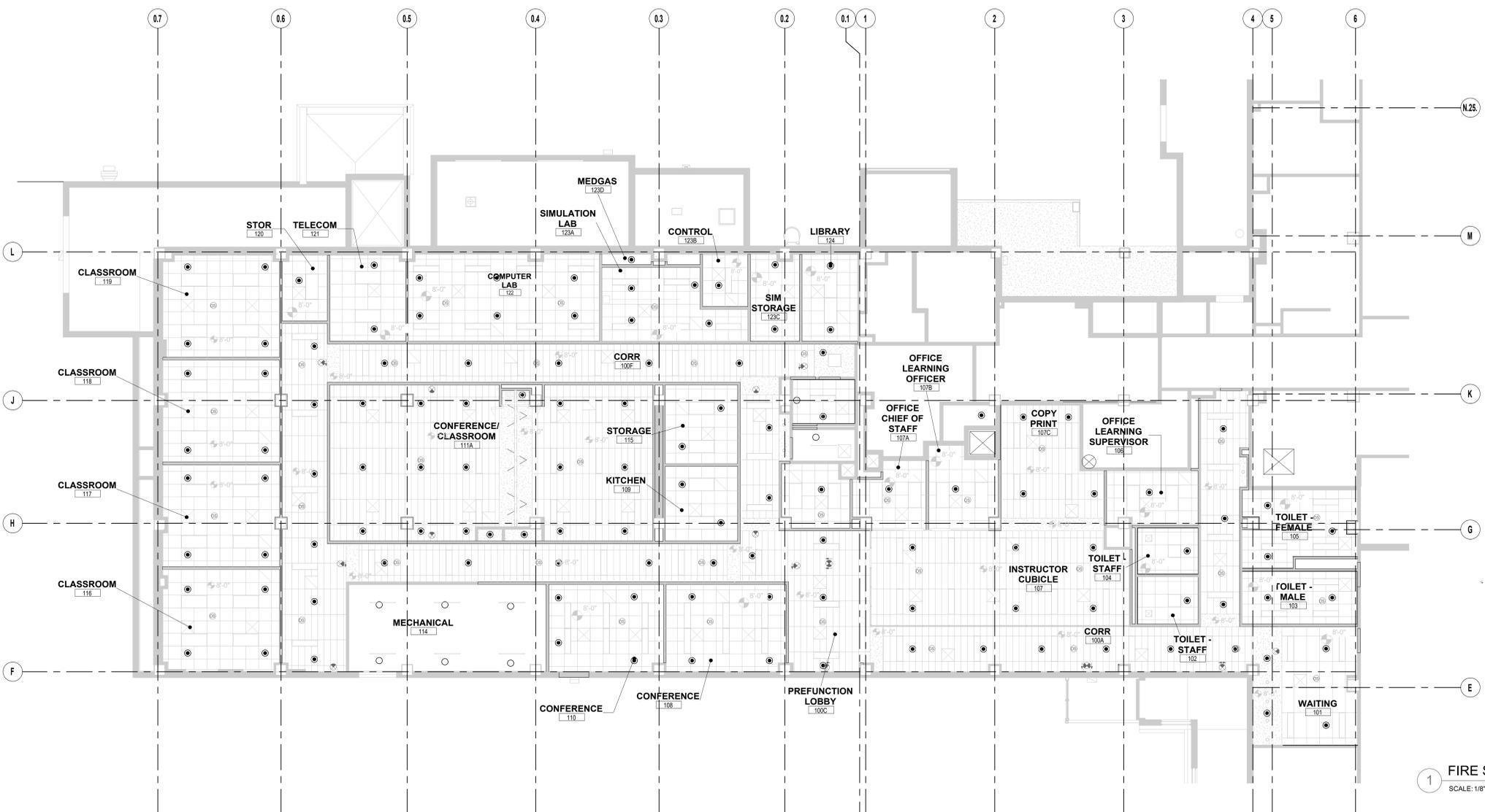
1. WORK FOR THIS BUILDING CONSISTS OF THE DESIGN AND INSTALLATION OF MODIFICATIONS TO AN EXISTING WET AUTOMATIC FIRE SPRINKLER SYSTEM IN ACCORDANCE WITH NFPA 13 REQUIREMENTS. THE SYSTEM IS HYDRAULICALLY DESIGNED TO PROVIDE 0.10 GPM PSF OVER 1500 SQ FT FOR LIGHT HAZARD.
