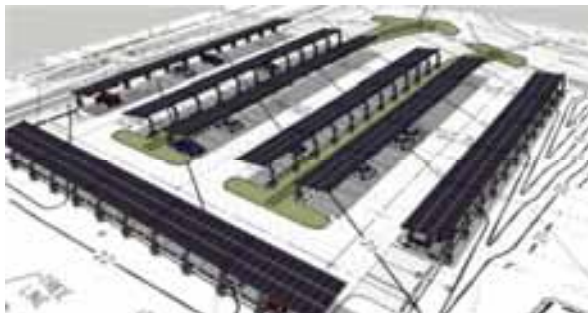
Photovoltaic array arranged to provide parking shade
