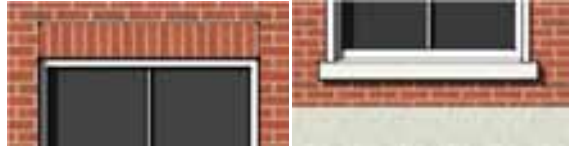
(Left) Example of window head using soldier coursing; (Right) Example of precast concrete sill
