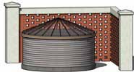
This above ground cistern is obscured from view with a traditional brick screen wall pattern that would be appropriate for most districts
