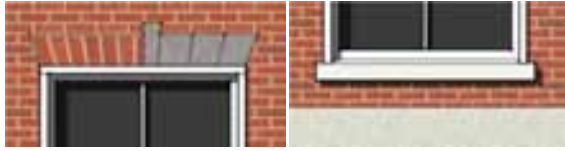
(Left) Example of jack arch using brick or precast concrete; (Right) Example of precast concrete sill
