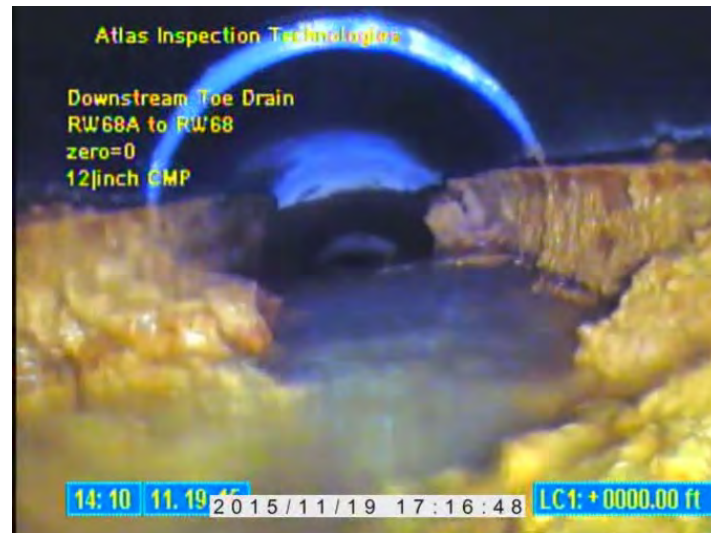
Figure 1-8: Left abutment relief well collector system RW-68A to T-outfall
