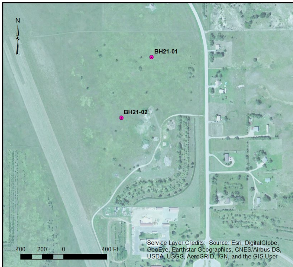
Figure 9: Borrow area soil boring locations BH21-01 and BH21-02 (north of project office)
