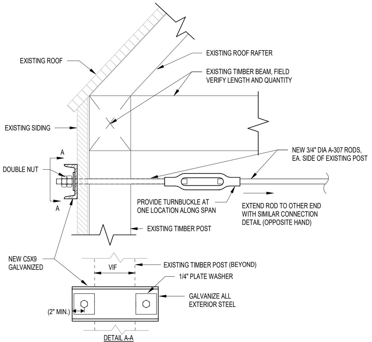
SCOPE OF REPAIR INCLUDES INSTALLATION OF PAIRS OF NEW 3/4" DIAMETER STEEL RODS SPANNING THE ENTIRE WIDTH OF THE EXISTING STRUCTURE AT FOUR LOCATIONS. THIS SKETCH SHOWS THE CONNECTION DETAIL FOR ONE PAIR OF STEEL RODS AT ONE SIDE OF THE STRUCTURE. INSTALL A TURNBUCKLE ALONG THE SPAN OF EACH ROD TO ALLOW INSTALLATION AND SUFFICIENT TENSIONING.
