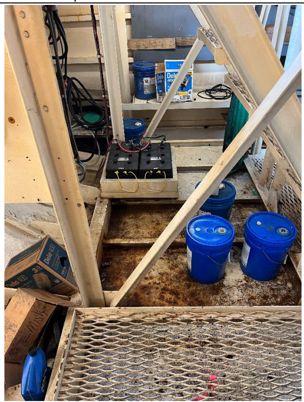
Areas of rust in generator/aft compartment
