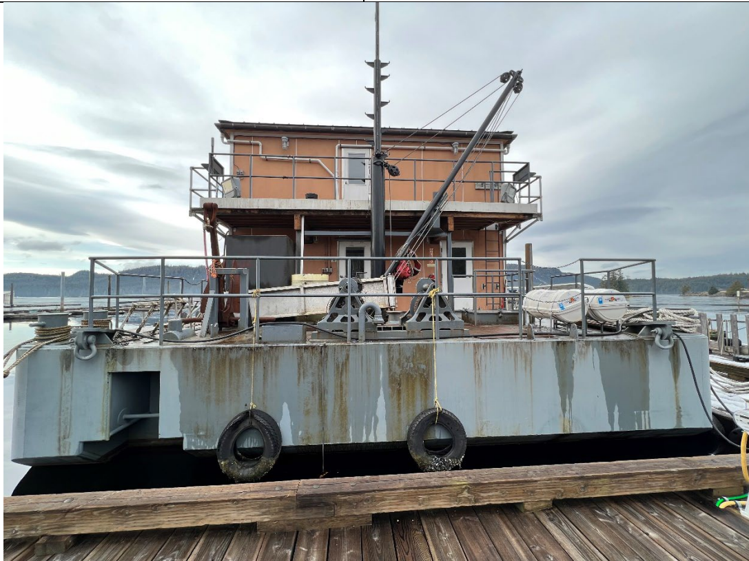
Forward – Visible 1000 lb anchor, zodiac liferafts, two winches, crane/boom and mast
