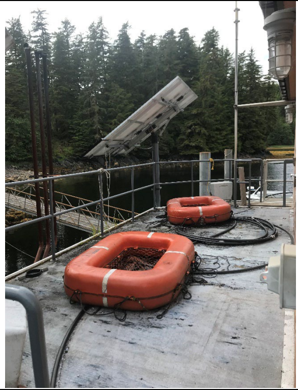
Aft Upper Exterior Deck to be replaced with aluminum decking.
