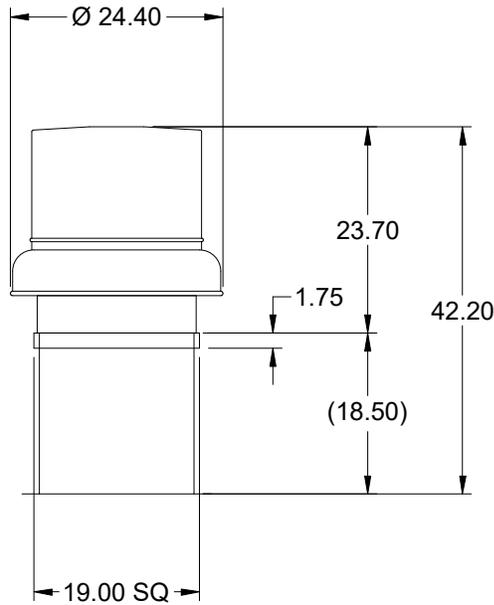
DUCT DIMENSIONS ARE LARGEST POSSIBLE DUCT TO FIT THROUGH CURB.
