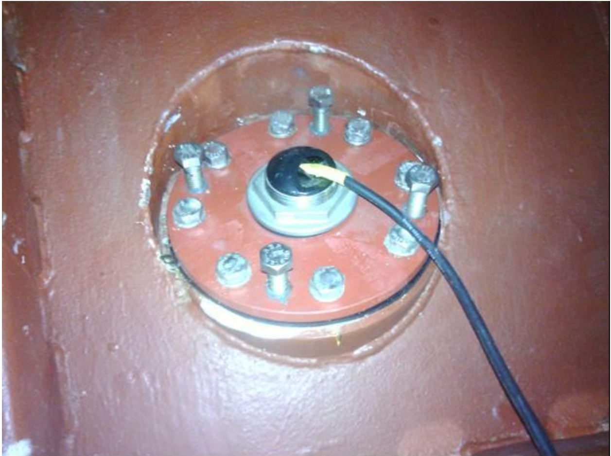
FIGURE 1. INTERIOR HULL ADAPTER PLATE
