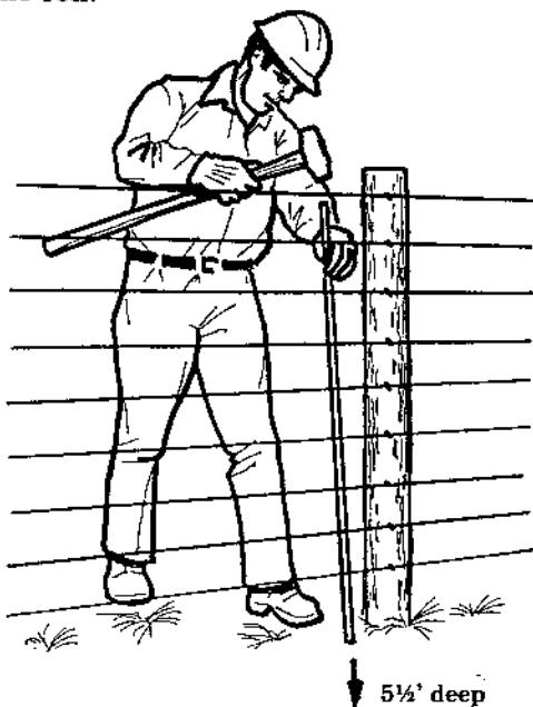
Installing a ground rod.
