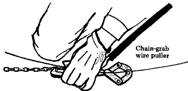
Tightening guide wire.
