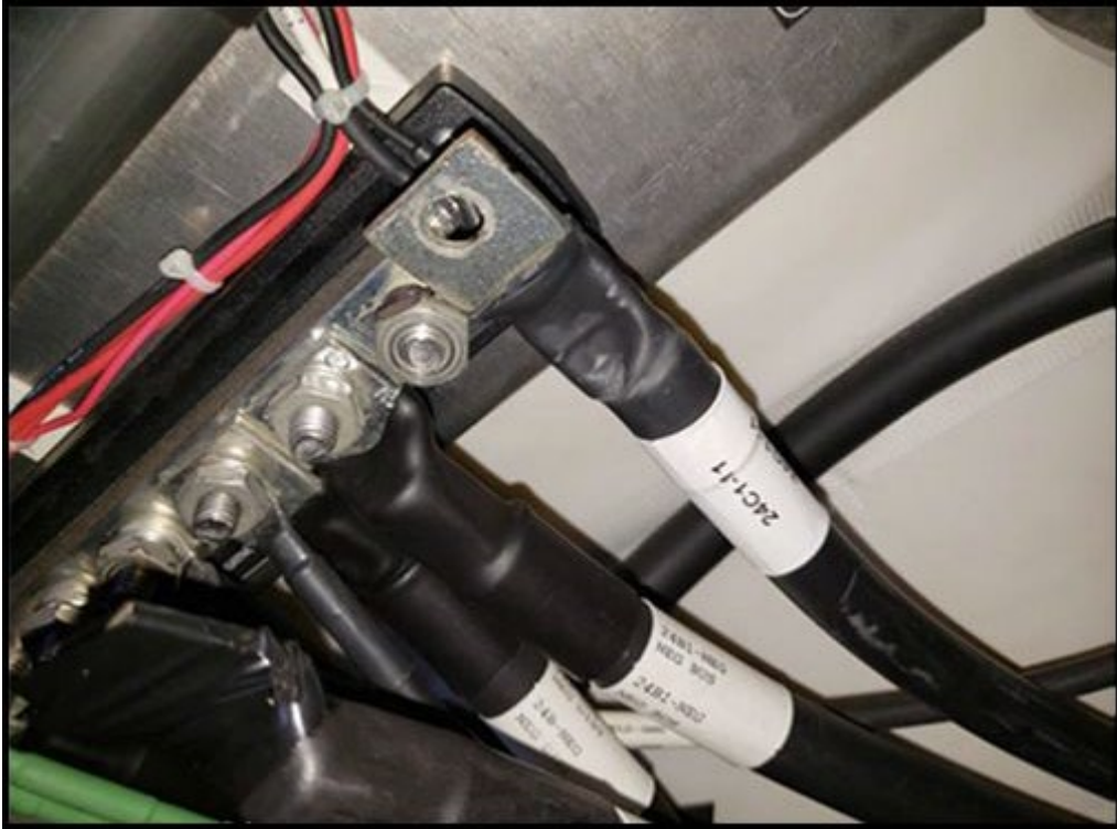
FIGURE 5. NEGATIVE BATTERY CABLE
