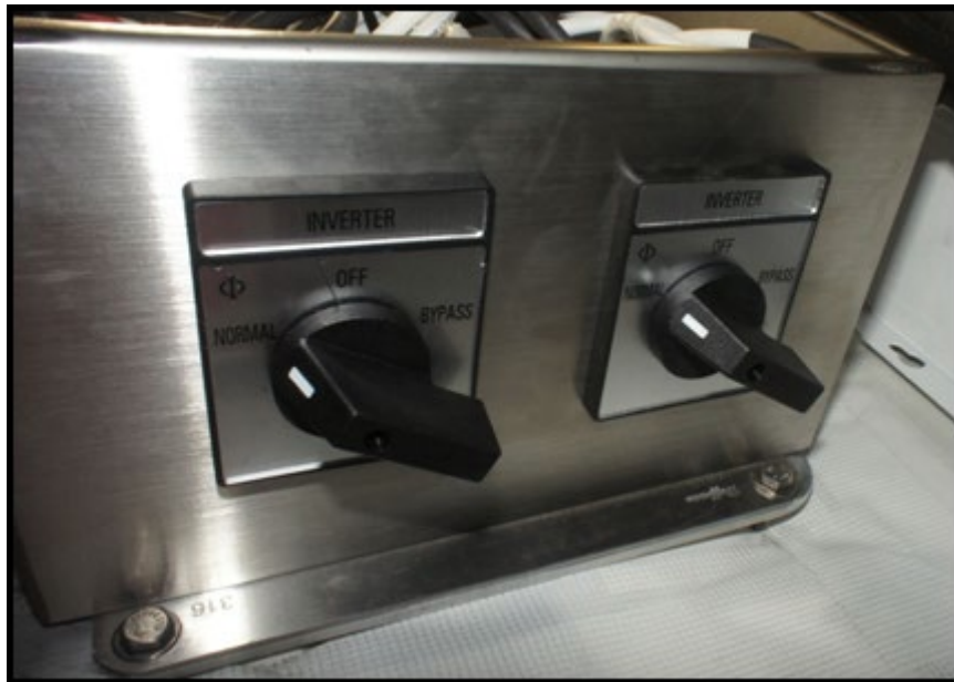
FIGURE 3. INVERTER BYPASS SWITCH
