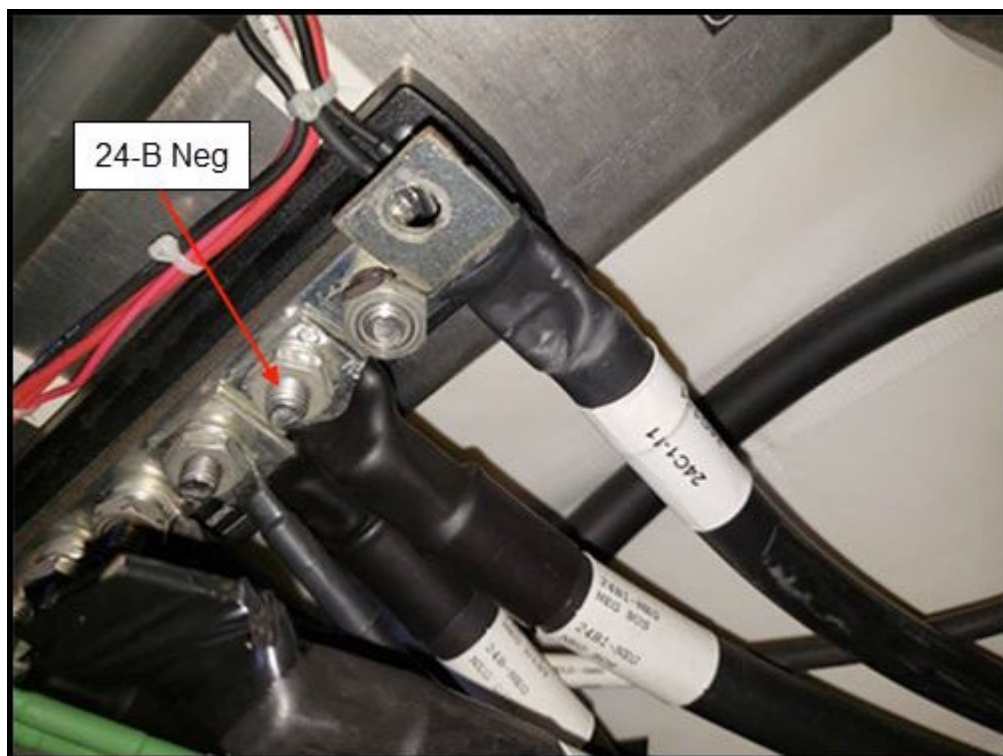
FIGURE 9. HULL GROUND
