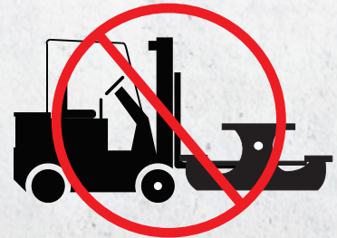
Unacceptable Method!! DO NOT ATTEMPT TO LIFT OR MOVE UNDER SEATS!
