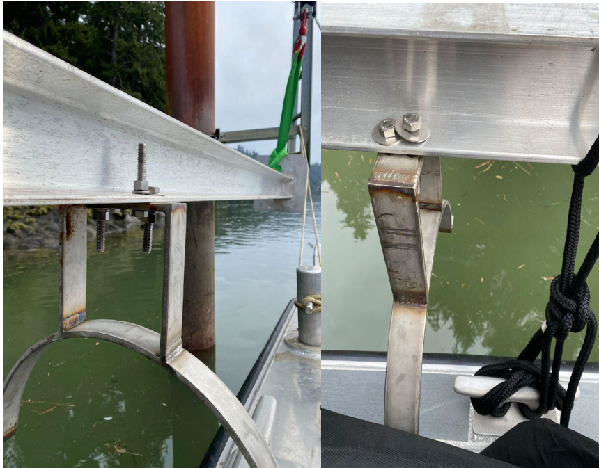
Figure 2 Bracket front section mounted on I-Beam - this would remain attached to the I-beam
