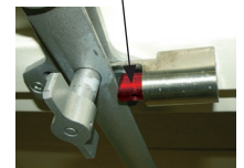
STOP SHOWN WHEN DOOR IS FULLY OPENED
