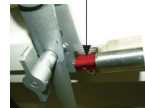
STOP SHOWN BEFORE DOOR IS FULLY OPENED
