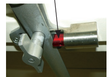
STOP SHOWN WHEN DOOR IS FULLY OPENED
