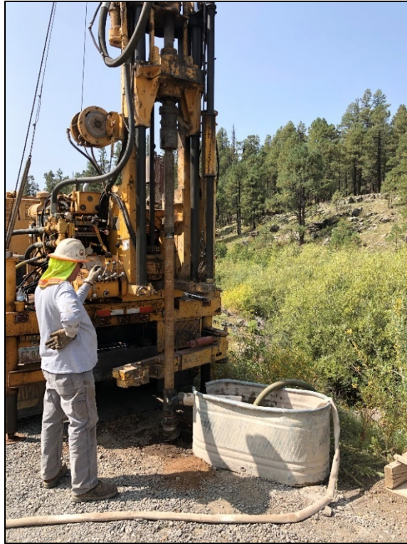
Photo 22: Rock Coring, Boring BH20-02
