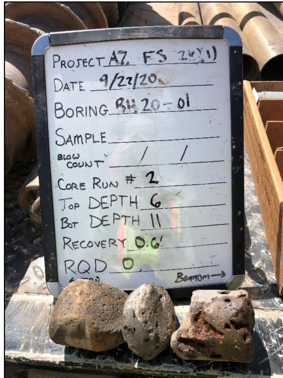
Photo 16: Core Run #2, Boring BH20-01
