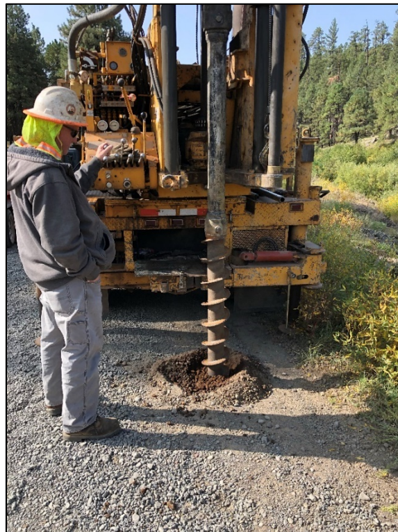
Photo 21: Hollow Stem Auger Drilling, Boring BH20-02
