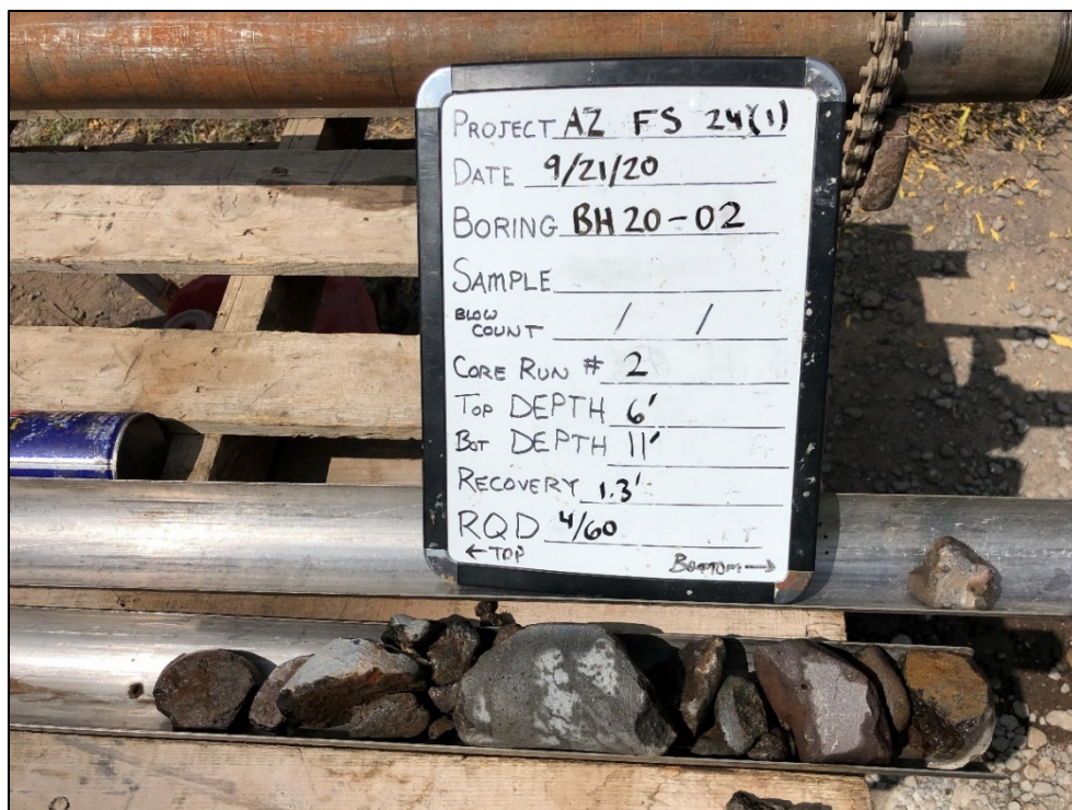
Photo 24: Core Run #2, Boring BH20-02
