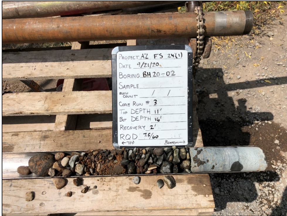
Photo 26: Core Run #3, Boring BH20-02
