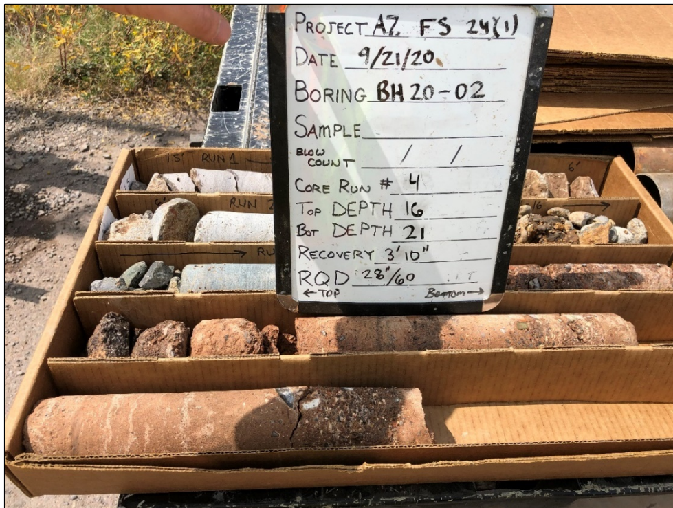
Photo 27: Core Run #4, Boring BH20-02
