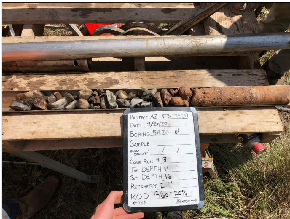
Photo 17: Core Run #3, Boring BH20-01
