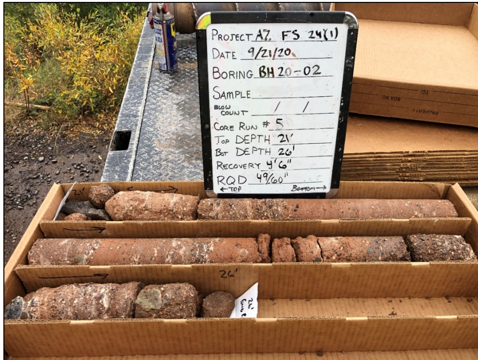
Photo 28: Core Run #5, Boring BH20-02
