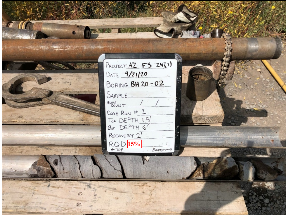
Photo 23: Core Run #1, Boring BH20-02
