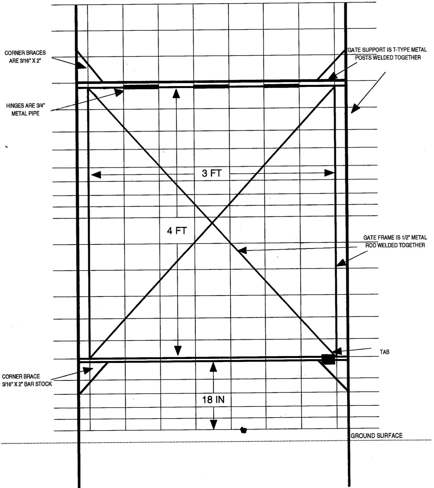
COVER GATE FRAME WITH PIECE OF FENCING WIRE
