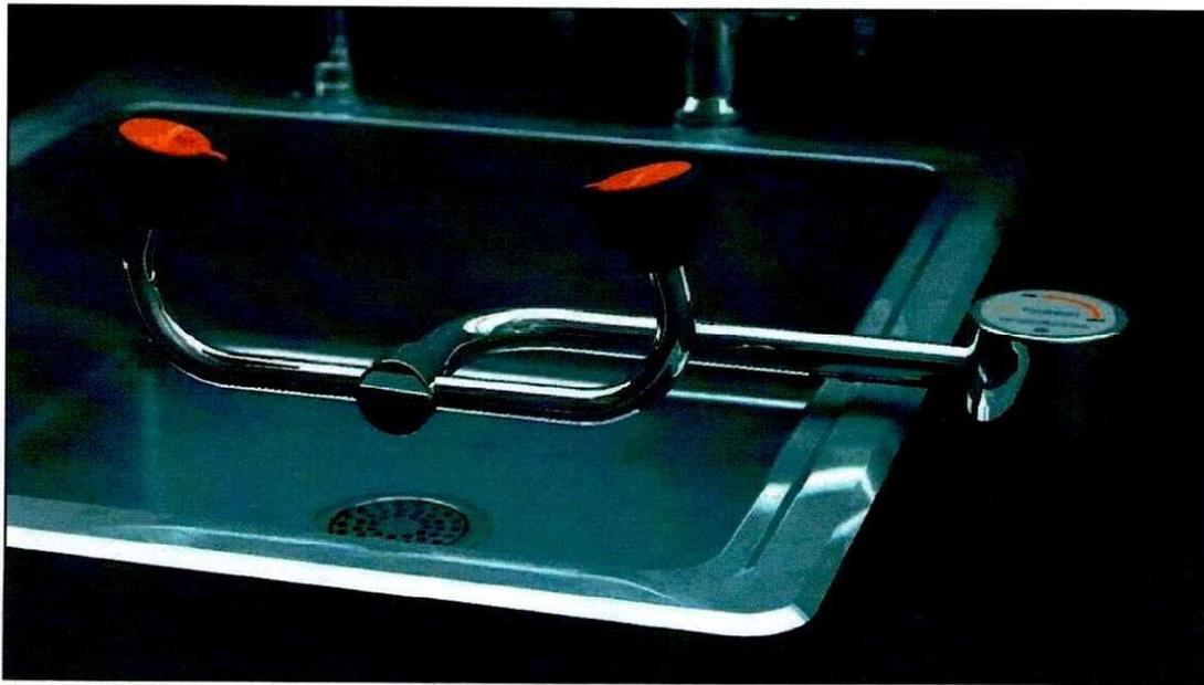
**Application:** AutoFlow™ eyewash for mounting next to sink. Swinging the spray head assembly horizontally out over the sink activates the water flow. The unit remains in operation until the spray head assembly is swung back into the storage position, closing the valve.
