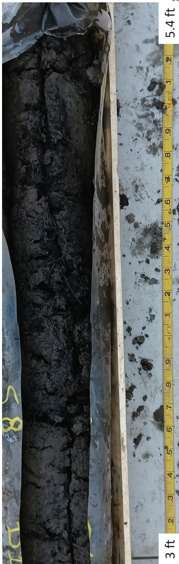
S8: 0-5.4 ft: dark brown, SILT and leaf material/organic debris
