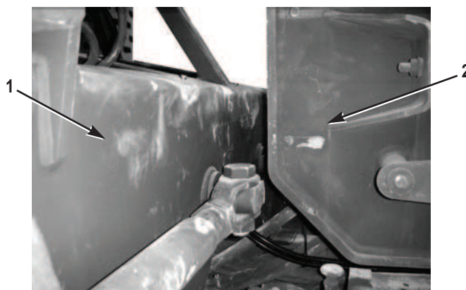
Figure 16. Distance Between Stowage Assembly and Hook Arm.
