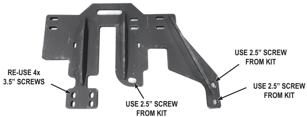
Figure 1. Assembly Guide, Driver Side.
