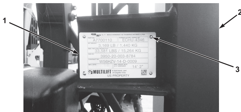
Figure 47. Data Plate Installation.
