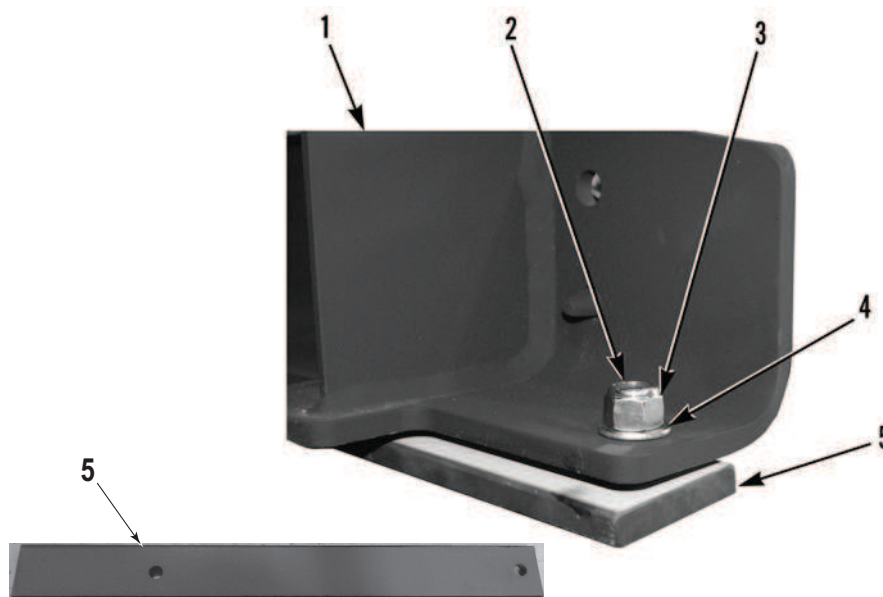
Figure 6. PLS A1 Stowage Assembly Spacers.
