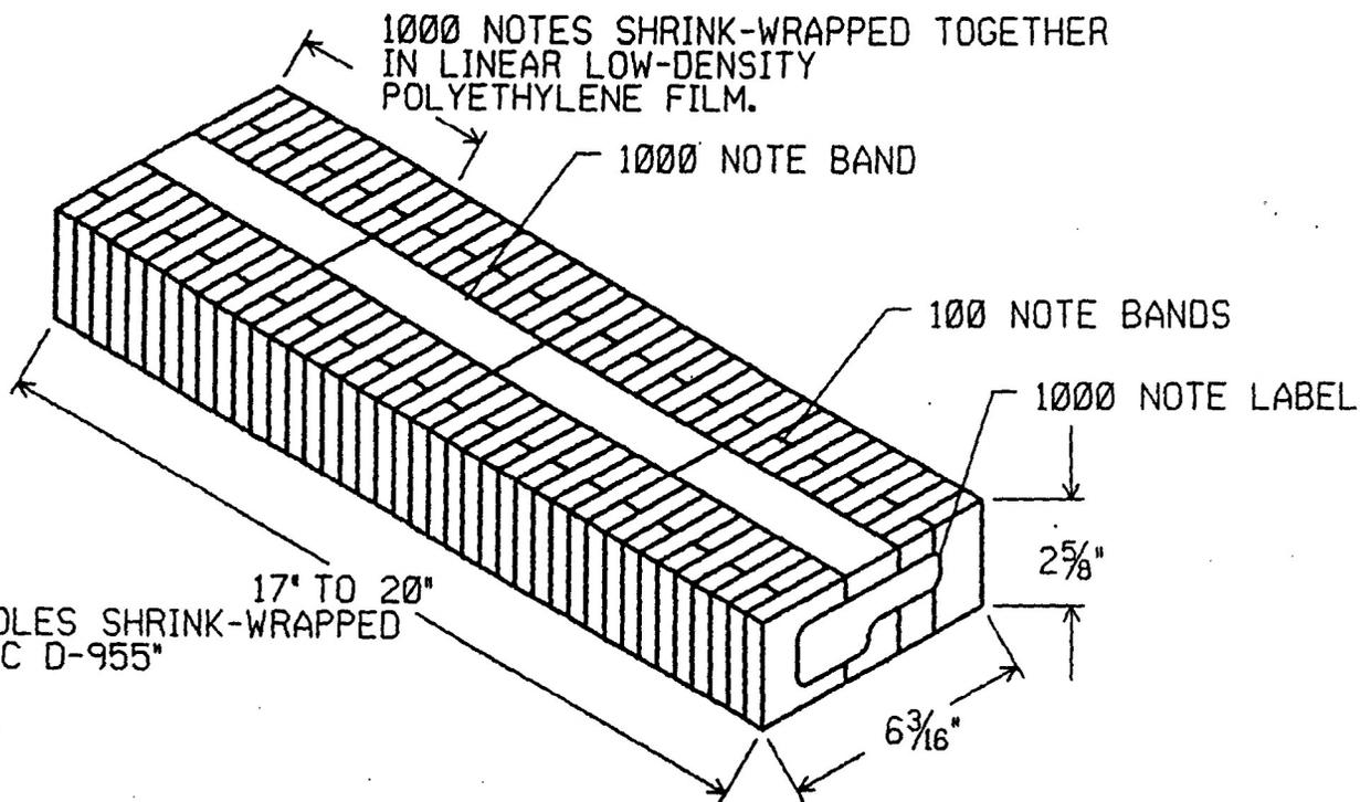
FOUR 1000 NOTE BUNDLES SHRINK-WRAPPED TOGETHER IN "CRYOVAC D-955" OR EQUIVALENT FILM.
