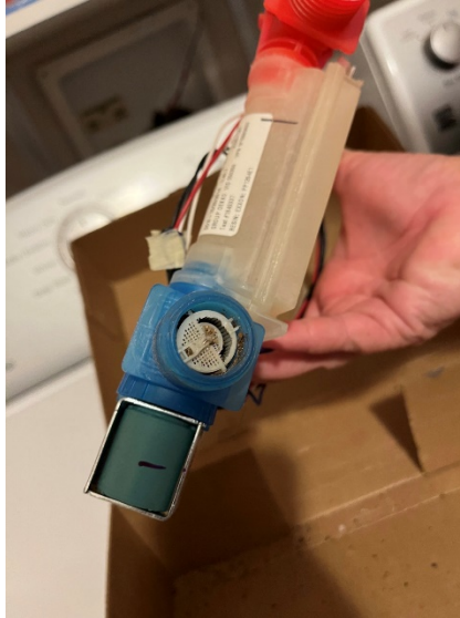
Replaced Washer Part with sediment
