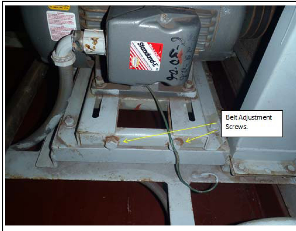
FIGURE 1. DRIVE BELT ADJUSTING SCREWS
