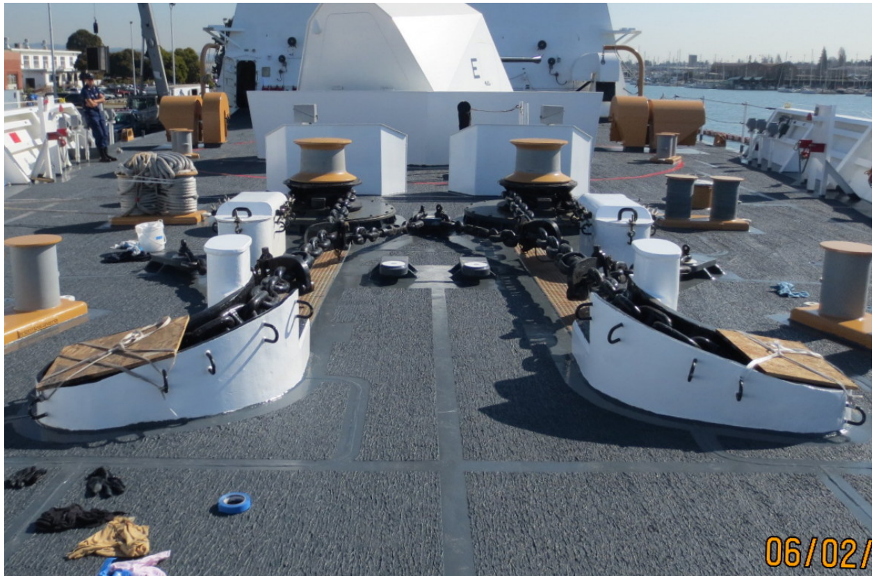
FIGURE 1: ANCHOR WINDLASS
